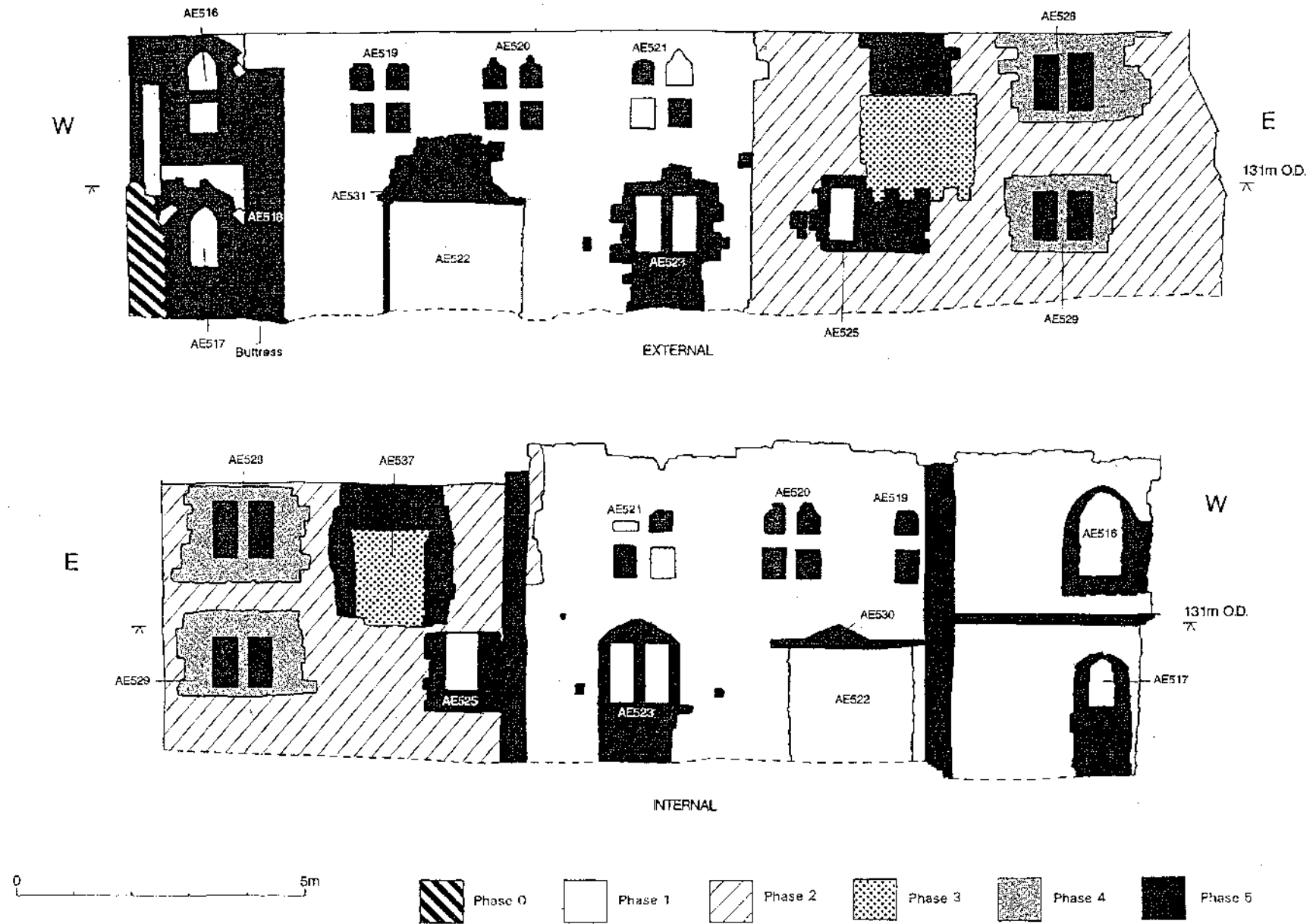
Fig. 6. Structure 1, phasing of south wall.
