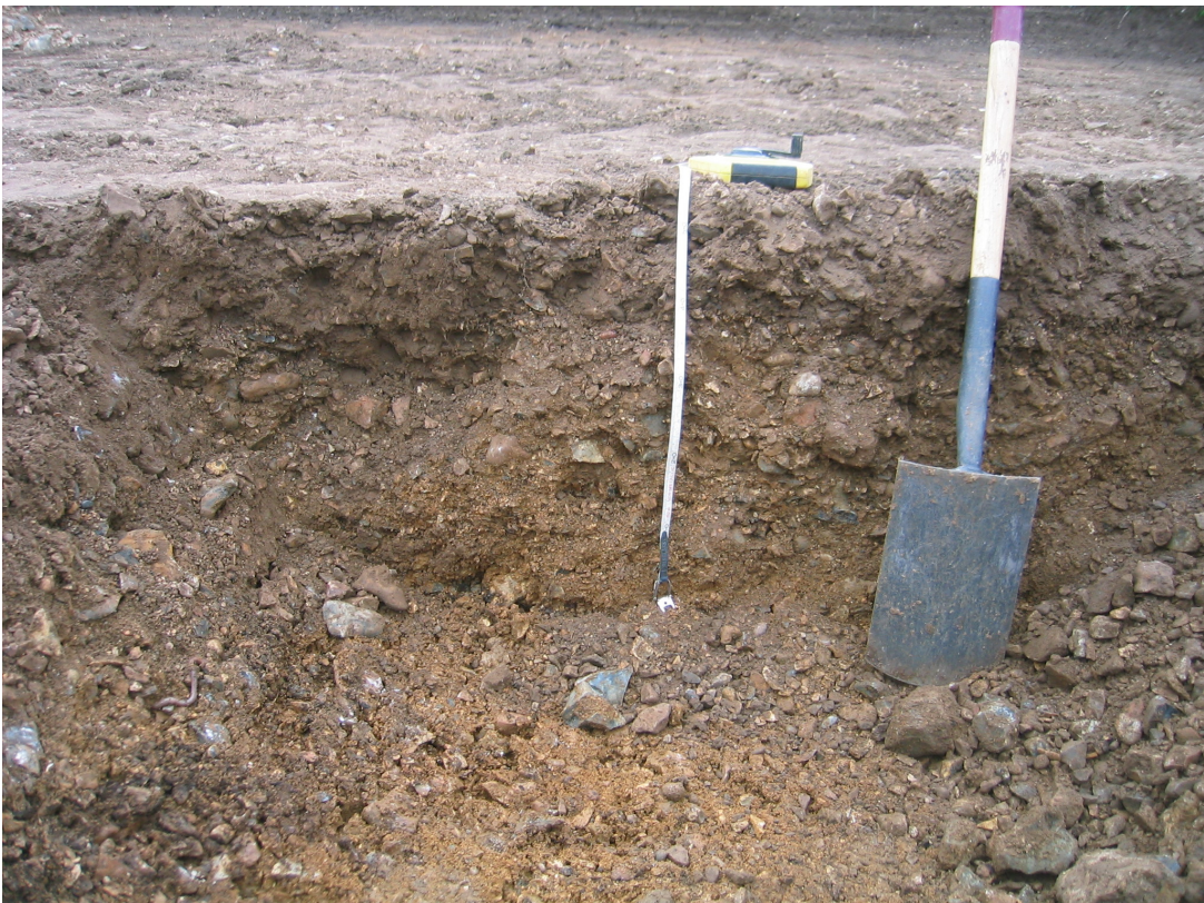
Figure 5: Trial Pit 2, located c. 25m west of Trial Pit 1 towards the valley sides. The stratigraphy is predominantly composed of colluvial sands and gravels.
