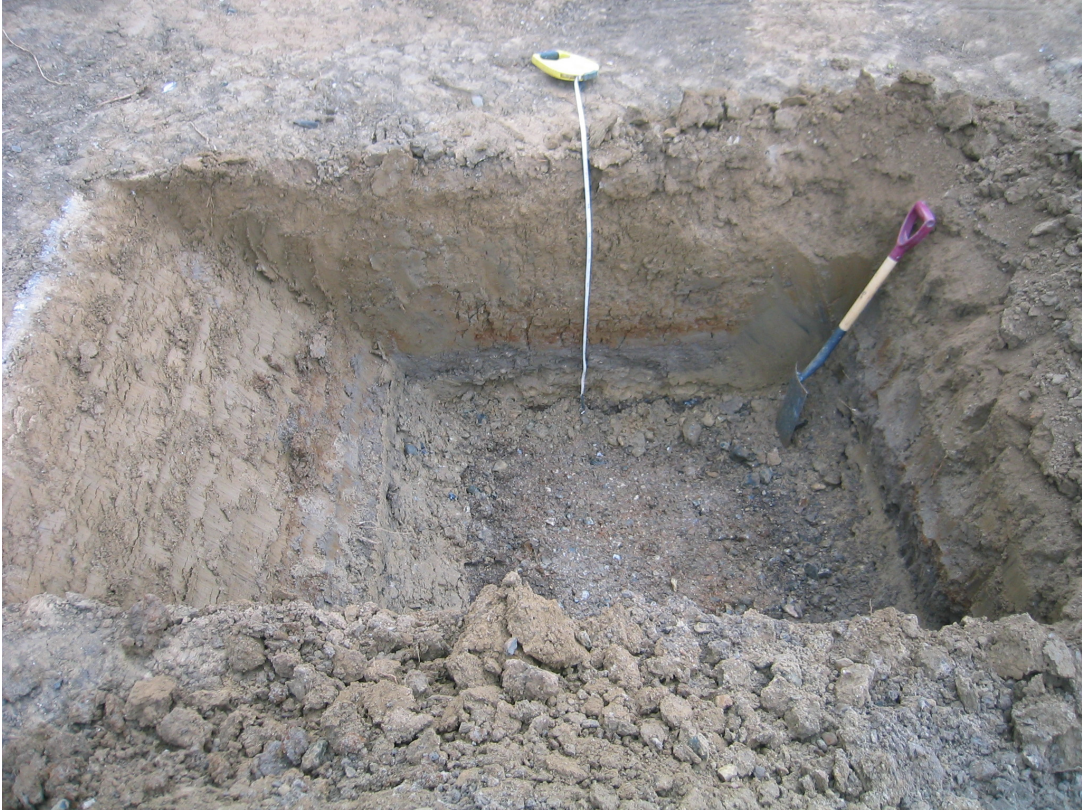
Figure 4: Trial Pit 1, located proximal to the River Lark. Comprised of c. 0.80m of alluvial clays and silts underlain by basal sands and gravels.
