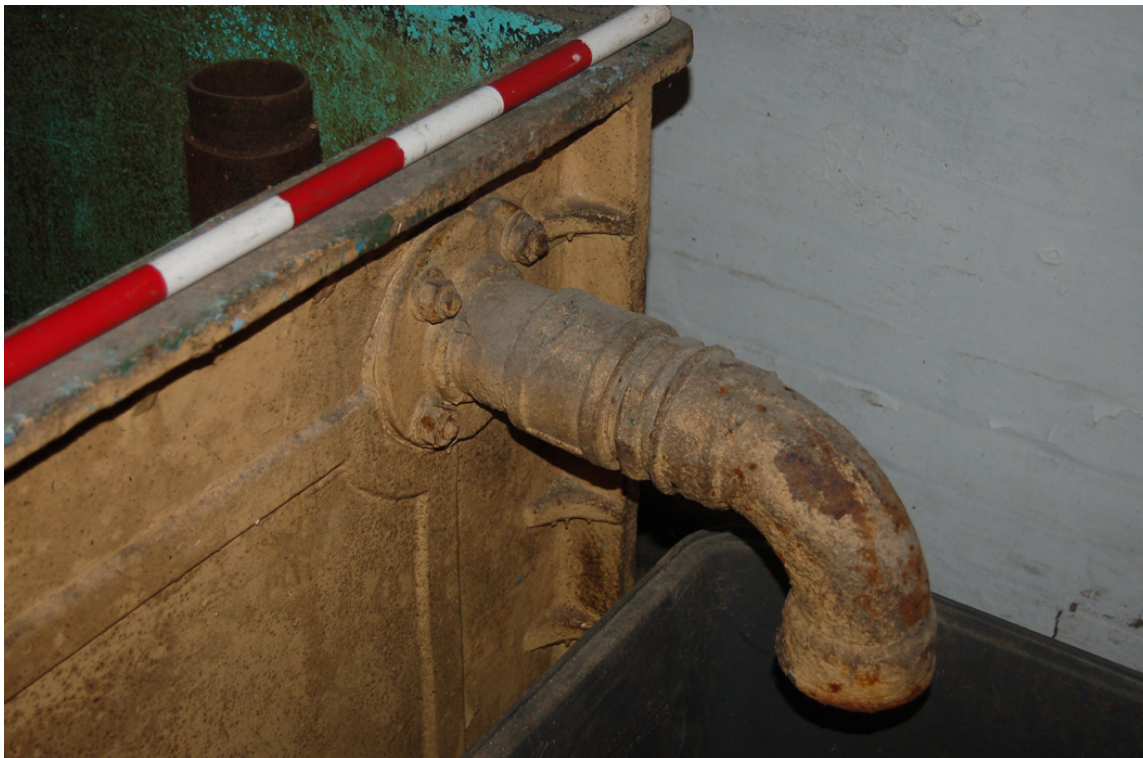
Plate 28: Barley intake range, [3F01]; detail of steeping vessel - overflow pipe.
