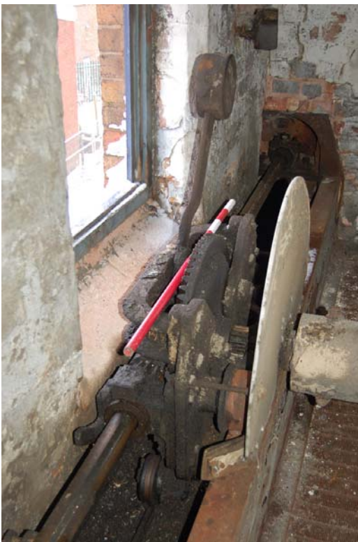
Plate 70: Kiln turner mechanism.
