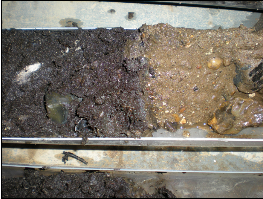
Plate 1: Core 9: Sandy organic silt overlying sands and gravels
