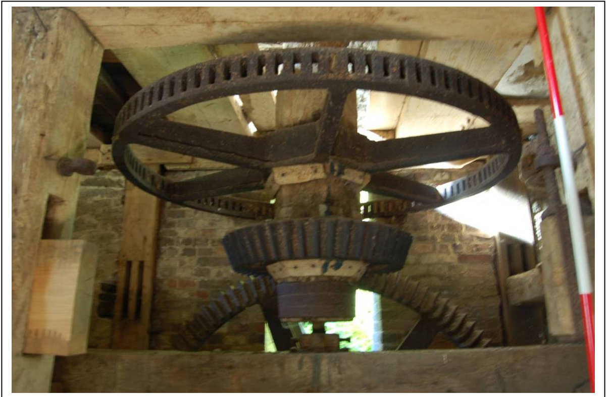
Plate 20: Spur wheel, west facing
