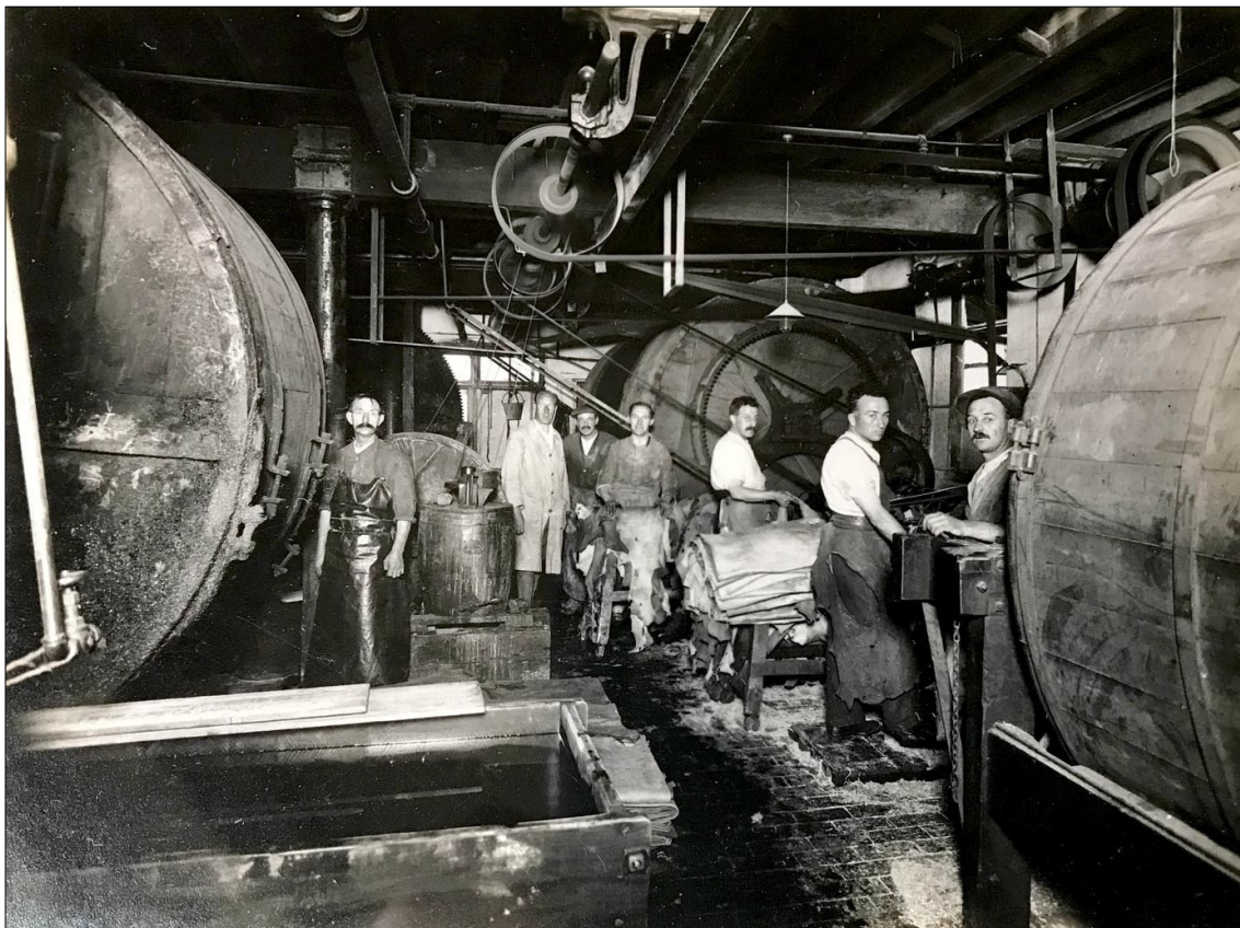
Figure 8. Dickens Brothers Leather Works, 1929 : fat liquoring and tanning processes (ground floor)
