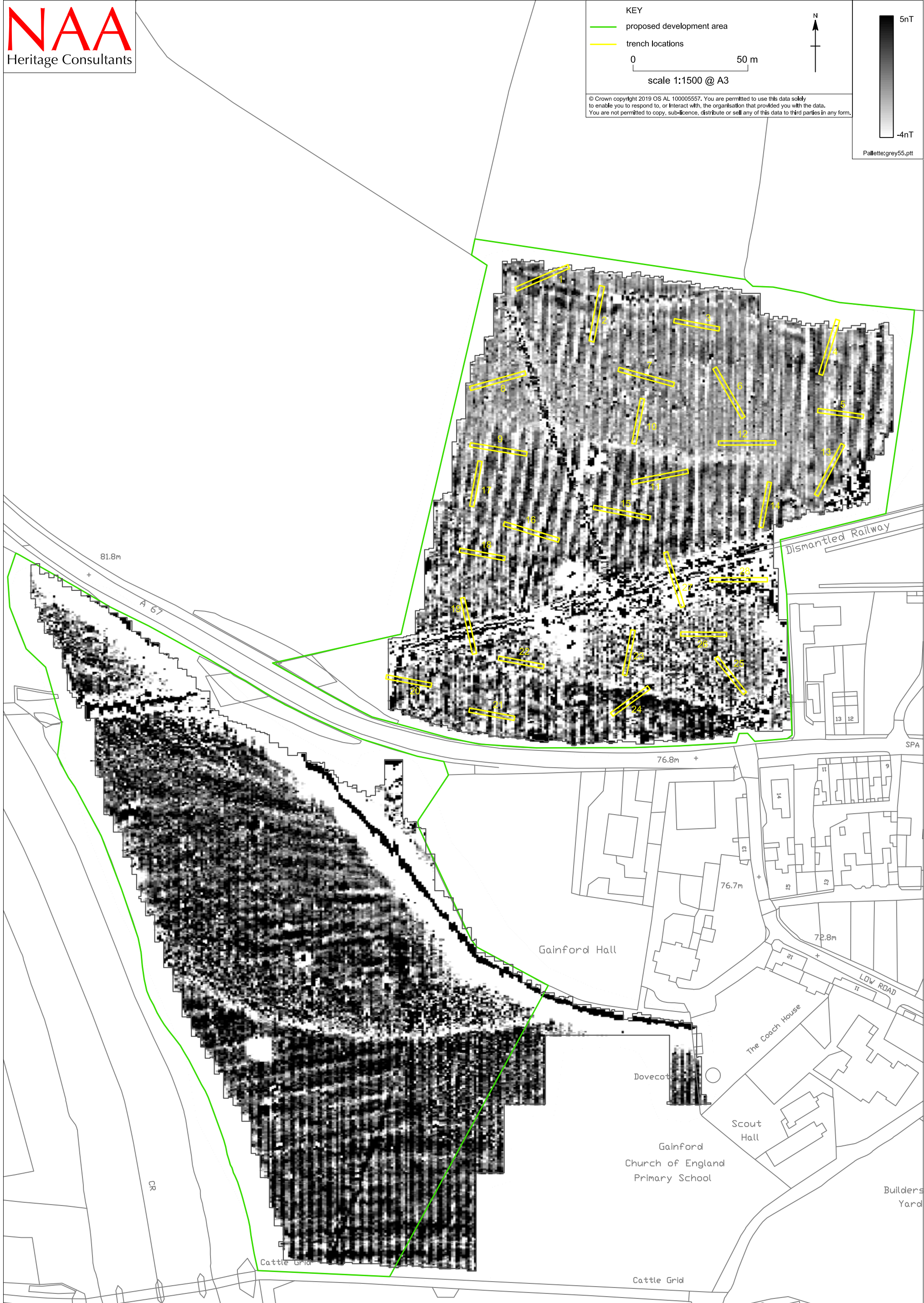
©NAA 2019 Land to the South of Spa Road, Gainford, County Durham: unprocessed greyscale plot of gradiometer survey results Figure 4
