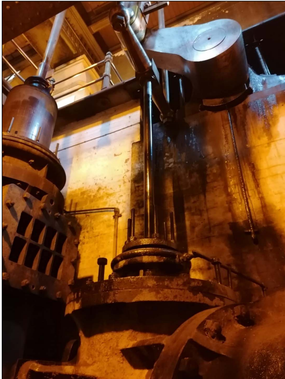
Plate 17: crankshaft (above) and 'town' (left) and 'river' (right) water pumps for the operational Edwardian beam engine
