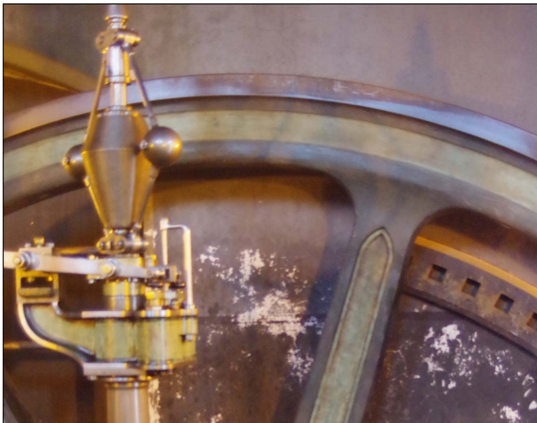
Plate 13: wall fixture relating to manual cranking of the flywheel in the Edwardian beam hall. Centrifugal governor visible on the left side of the photograph.
