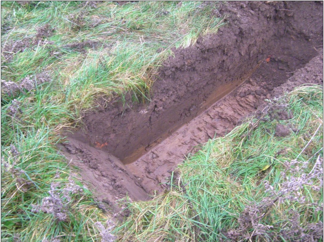
Plate 2: view of TP 60 showing imported modern material with CBM and concrete inclusions overlying natural glacial boulder clay, facing north-west.
