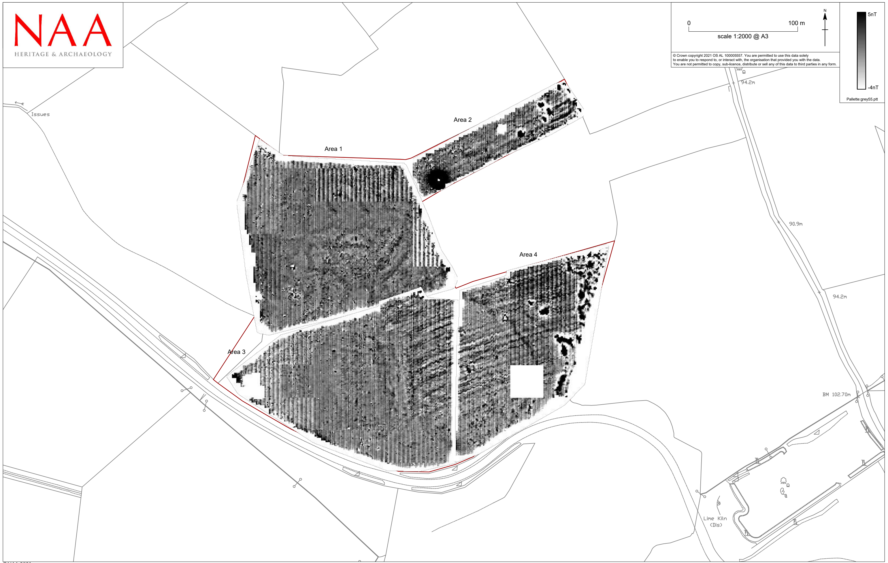
Field 3730, Tendley Quarry, Cumbria: unprocessed greyscale plot of gradiometer survey results
