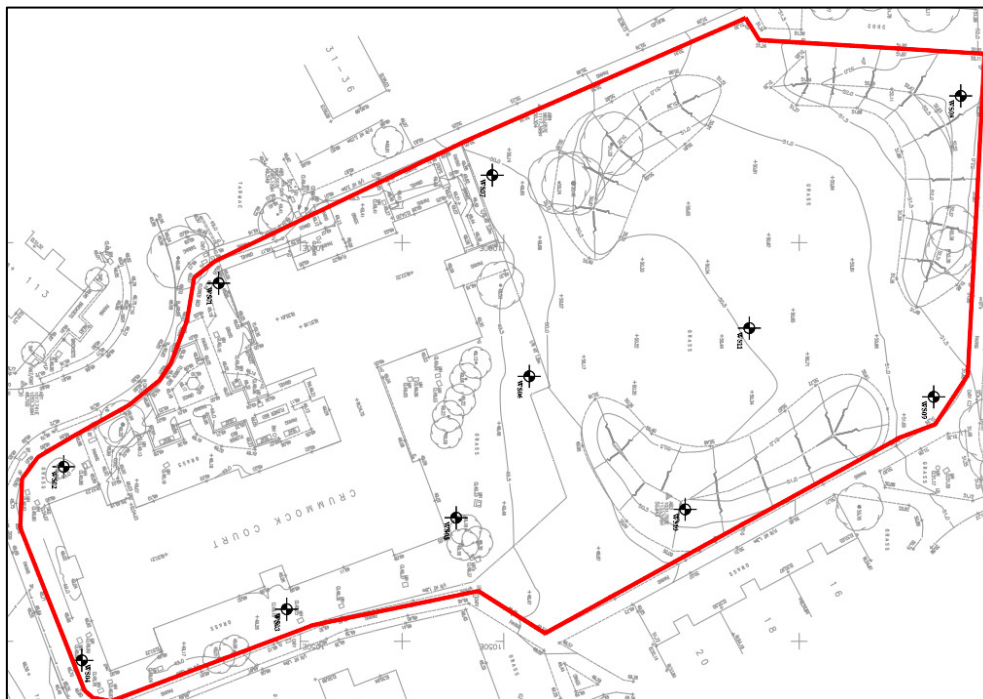
Illust 5: Plan showing earthwork mound and location of geotechnical test-pits and boreholes undertaken in 2009 3
