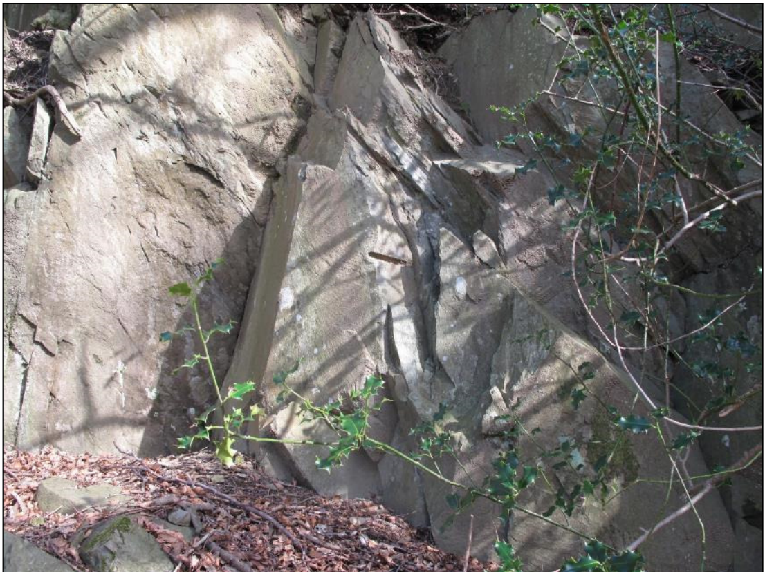
Plate 47: drill marks on a quarry face (23/001) in Bank Wood.
