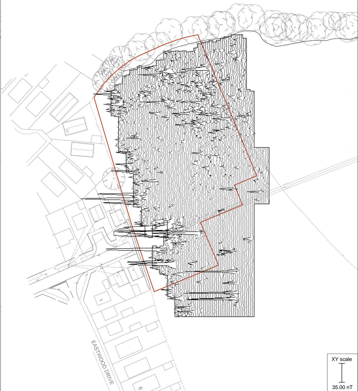
Hillside Road, Broughton, North Lincolnshire: unprocessed greyscale and XY-trace plots of gradiometer survey results
