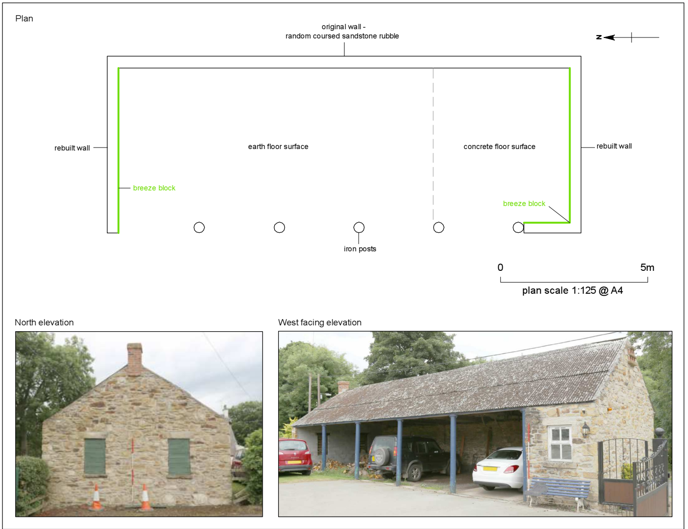
Witton Hall Farm, Witton Gilbert: Cart Shed, plan and elevations
