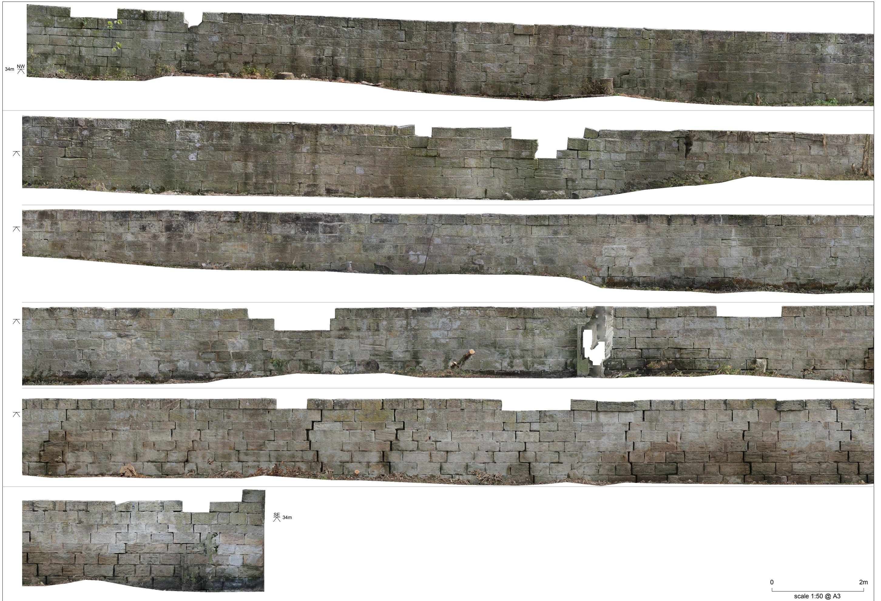
Church of Our Lady, Seaton Delaval: pre-intervention survey, west-facing elevation of west ha-ha wall.
