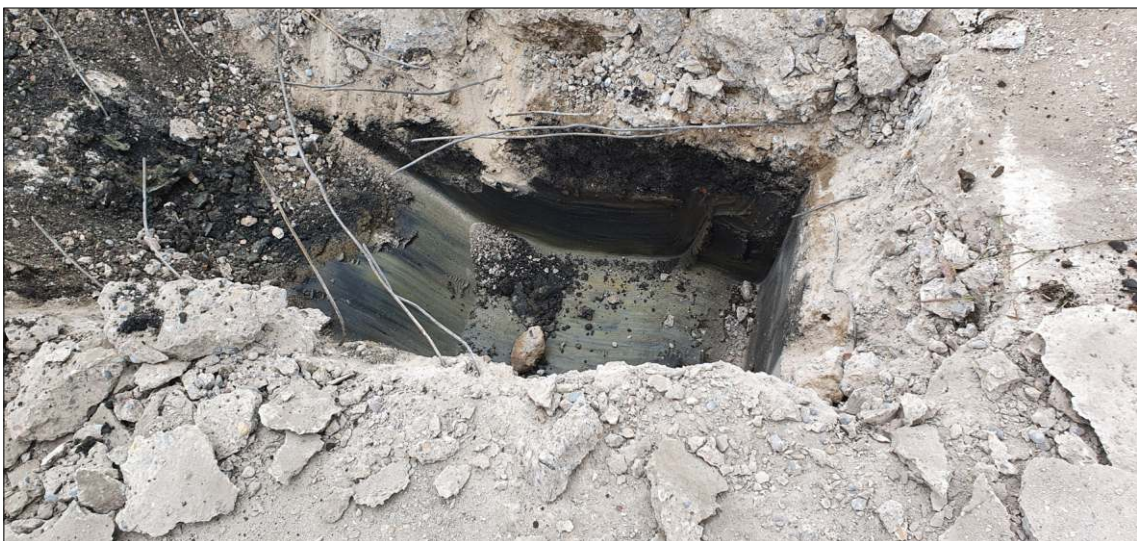
TVERF, Grangetown: DS12b showing industrial ash dumping directly over natural clay
