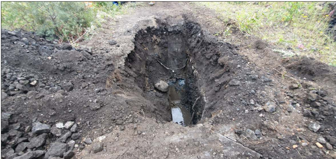
TVERF, Grangetown: DS9 showing depth of made ground over natural clay
