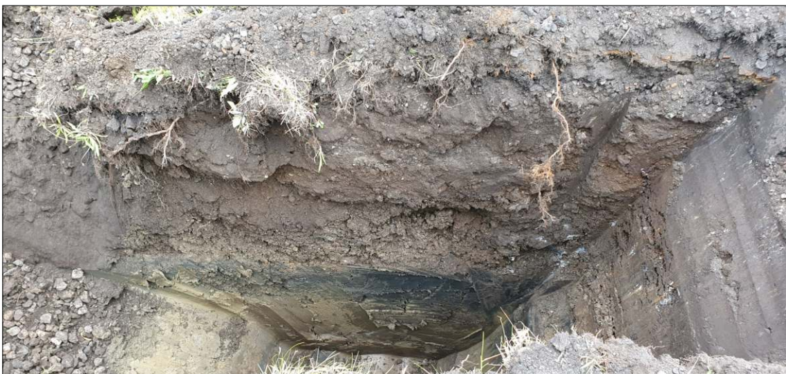
TVERF, Grangetown: TP12 showing industrial ash dumping directly over natural clay
