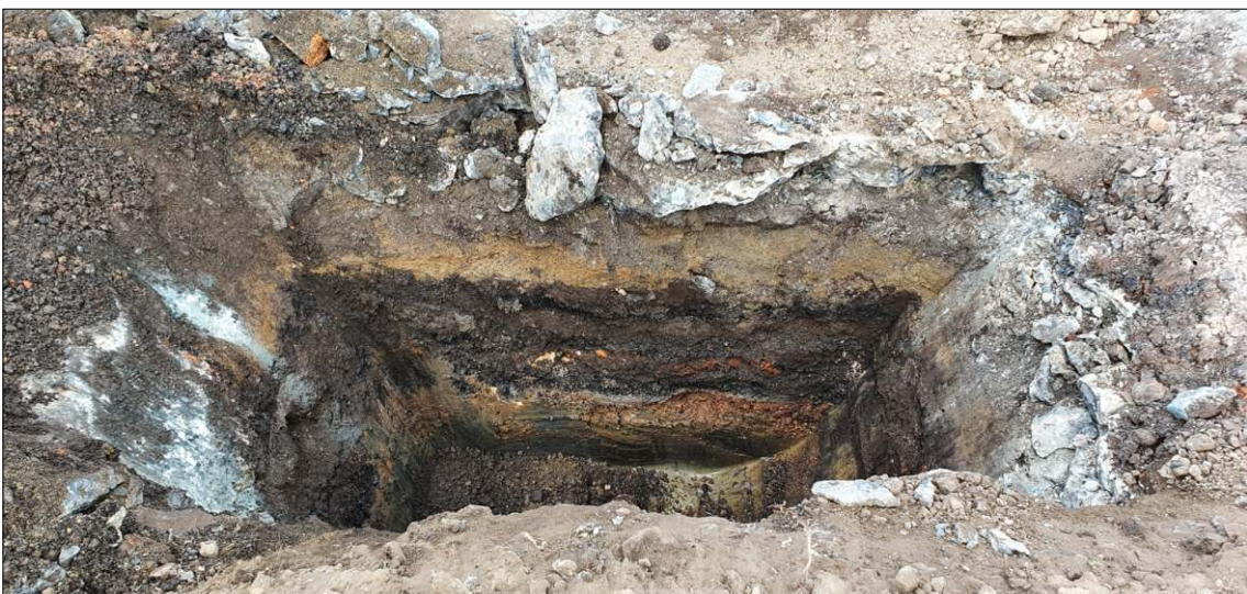
TVERF, Grangetown: DS4 showing industrial ash dumping directly over natural clay
