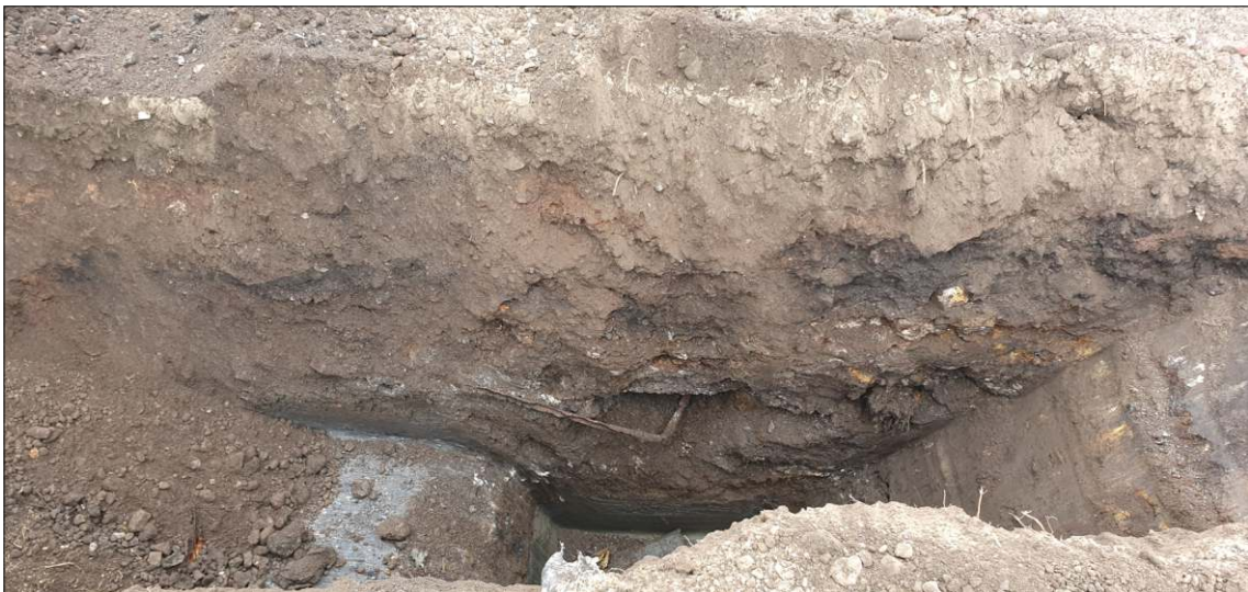
TVERF, Grangetown: BH1 showing industrial ash dumping directly over natural clay
