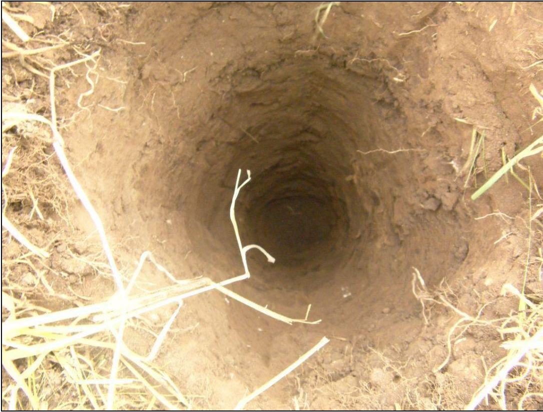
Plate 3. Borehole 1 starter pit on west side of River Torne, showing natural silty clay
