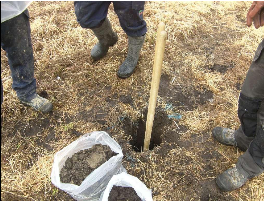
Plate 4. Clay and organic material from Borehole 2 starter pit on east side of River Torne
