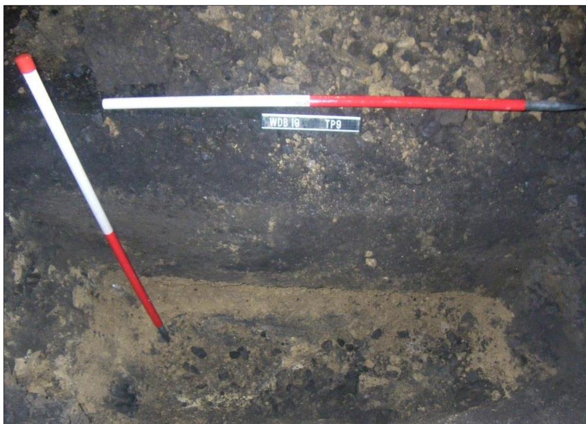
Plate 2. Typical trial hole profile showing crushed dolomite layer overlain by redeposited clay and grey road sub-base
