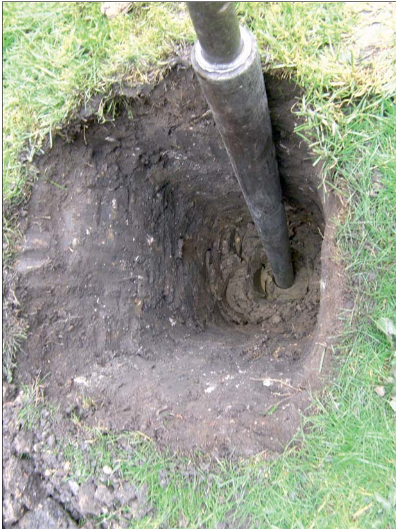
Union Terrace Geotechnical Investigation: Plate 2 soil profile in WS4
