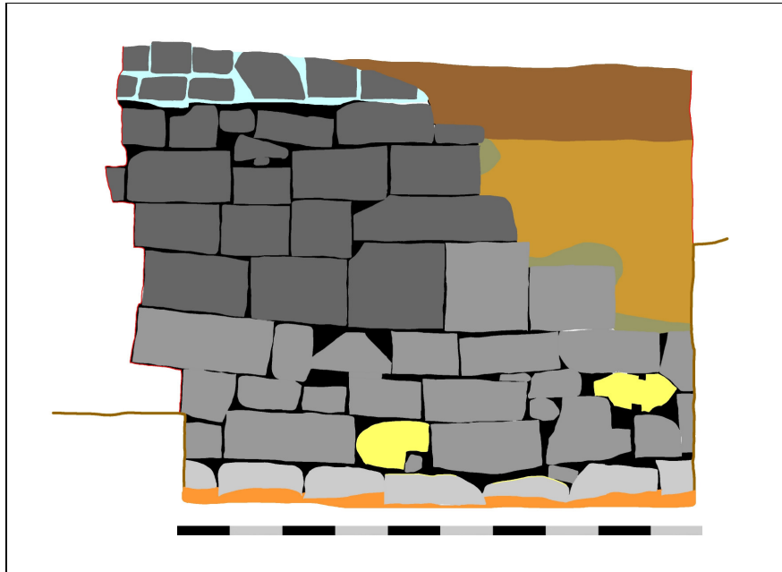
Fig.14 Elevation drawing of the ha ha wall in trench 4. The scale is 2m. Stonework in dark grey indicates the bulging out of the wall, that in light grey are the foundation stones and in yellow are Caen or Malm stone blocks. The orange at the base is the natural gravels, the brown at the top is modern topsoil, while beneath it in light brown is the natural sand, below this is the grey/green of the rubble behind the wall. At the top of the wall in light blue is the modern mortar.
