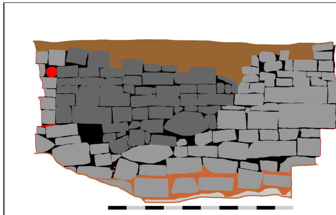
Fig.17 Elevation drawing of the ha ha wall in trench 5. The scale is 2m. Stonework in dark grey indicates the bulging out of the wall, that in light grey are the foundation stones. The brown at the base is roots, while the brown at the top is modern topsoil. The circular red is a modern pipe from the toilet block, while below it the rectangular red is a roof tile.
