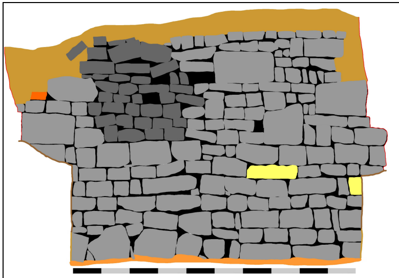
Fig.6 Elevation drawing of the ha ha wall in trench 1. The scale is 2m. Stones in dark grey indicate a bulging out of the wall, while those in yellow are Caen/Malm stone, with the red being a brick. The orange at the base is the natural gravel, while the brown above the wall is modern topsoil.
