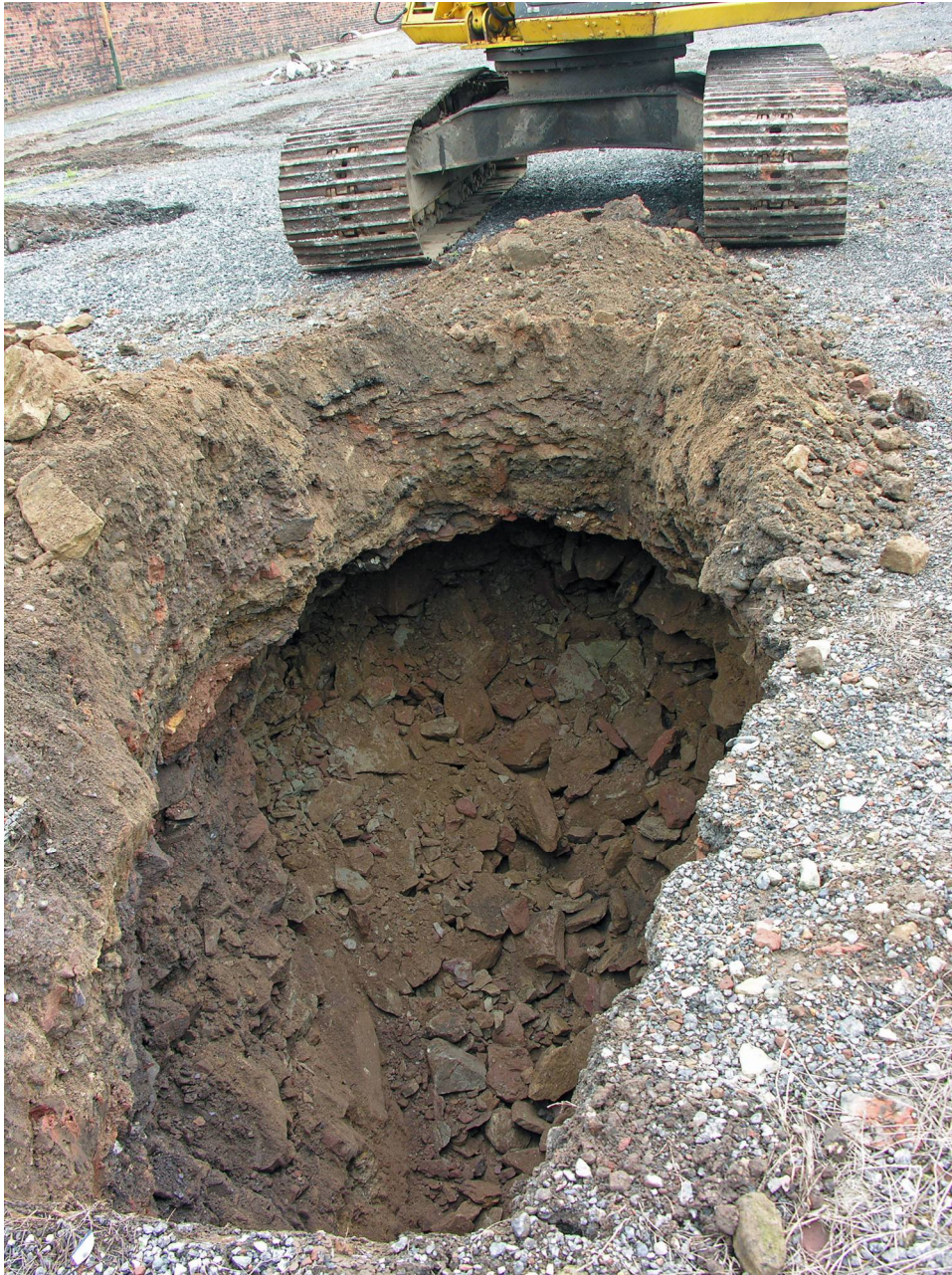
Plate 1. Test-pit 1 under excavation showing collapse of sides.
