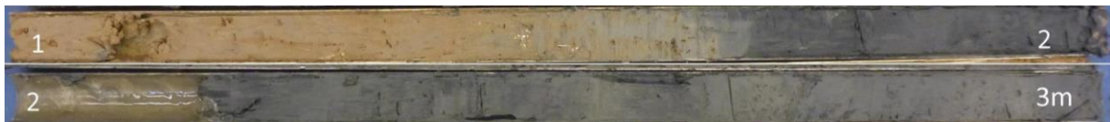
Figure 11. Oxidised deposits overlying the reduced deposits: very dark grey silt/clays in the upper right and lighter grey silt/clays in the core below. (1 to 3m bgl BH A).
