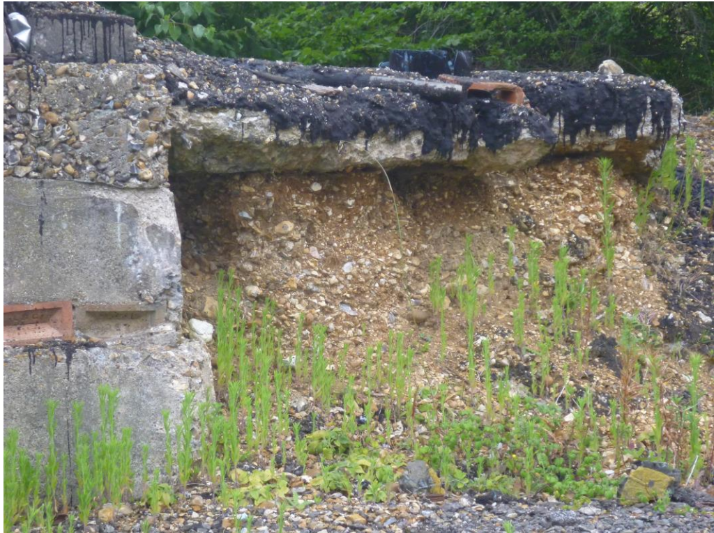
Figure 4 Outcrop of the Black Park Member in the old quarry overlain by concrete.
