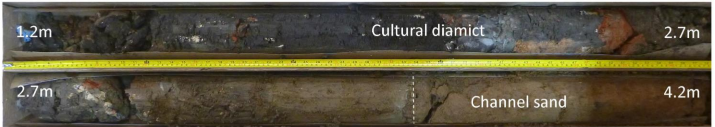
Figure 6. BH1 1.2–4.2m bgl showing the dark diamict containing cbm overlying channel sands.
