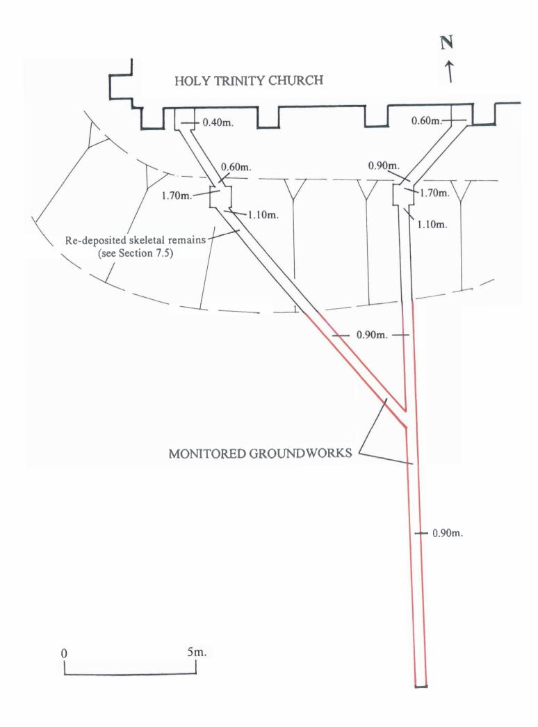
Figure 9: Groundworks location plan showing depths of excavation
