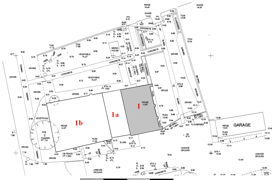
Figure 7 Ground plan of ‘Barn 1’ highlighting the 19 th century vehicle shed (1) in grey with the late-20 th century cement-block lean-to (1a) and workshop (1b) adjoining on the west.
