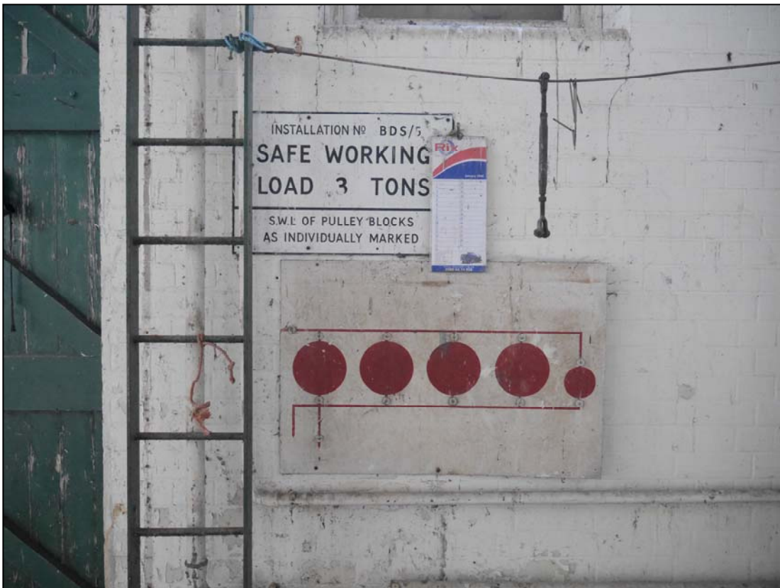
Plate 66. Fuel tank status diagram, also a gantry crane weight limit sign
