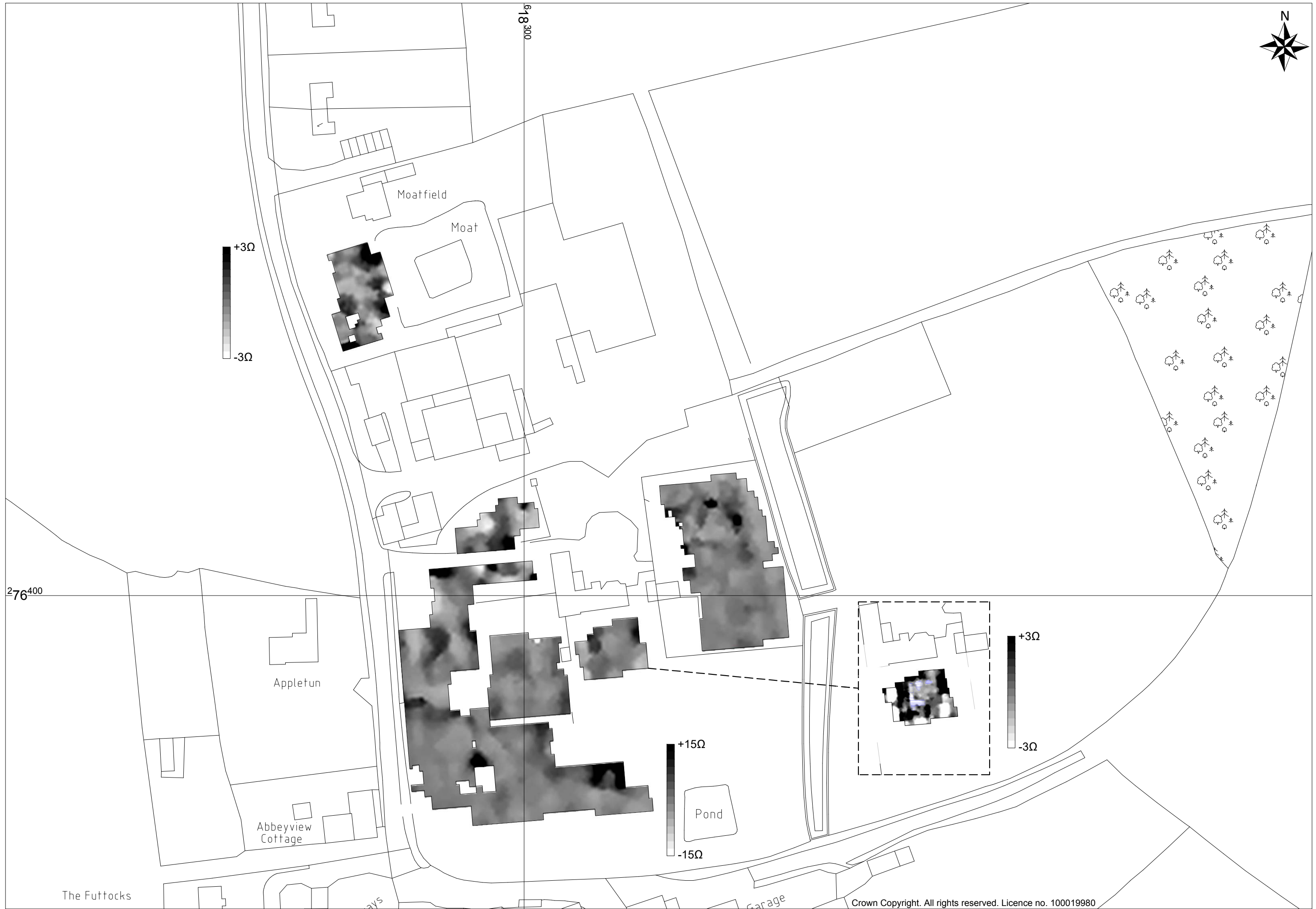
Fig. 10a. Combined surveys, processed earth resistance meter greyscale plots, showing detailed earth resistance meter insert
