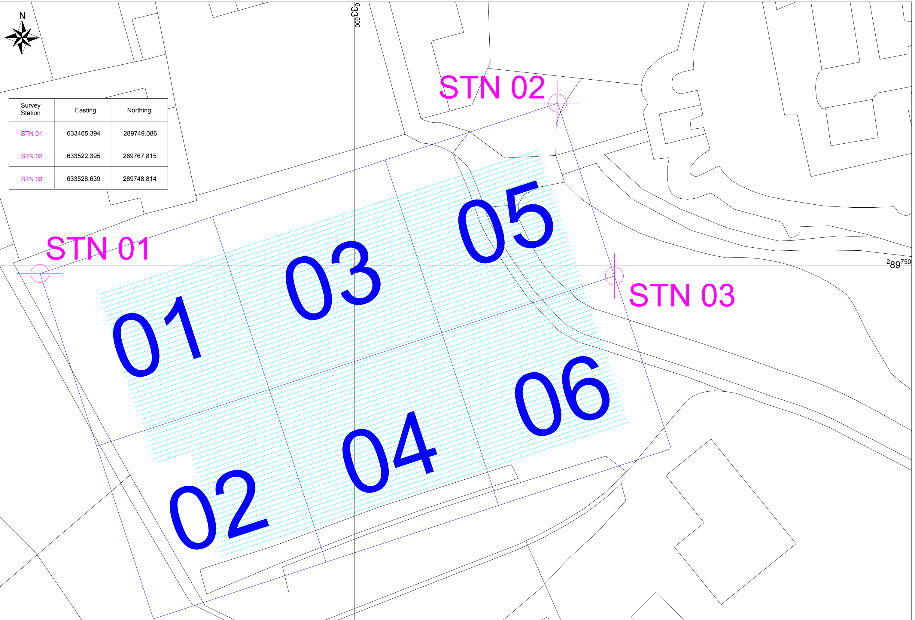
Figure 3. Survey grid (dark blue), GPR traverses (cyan) & georeferencing information (magenta)
