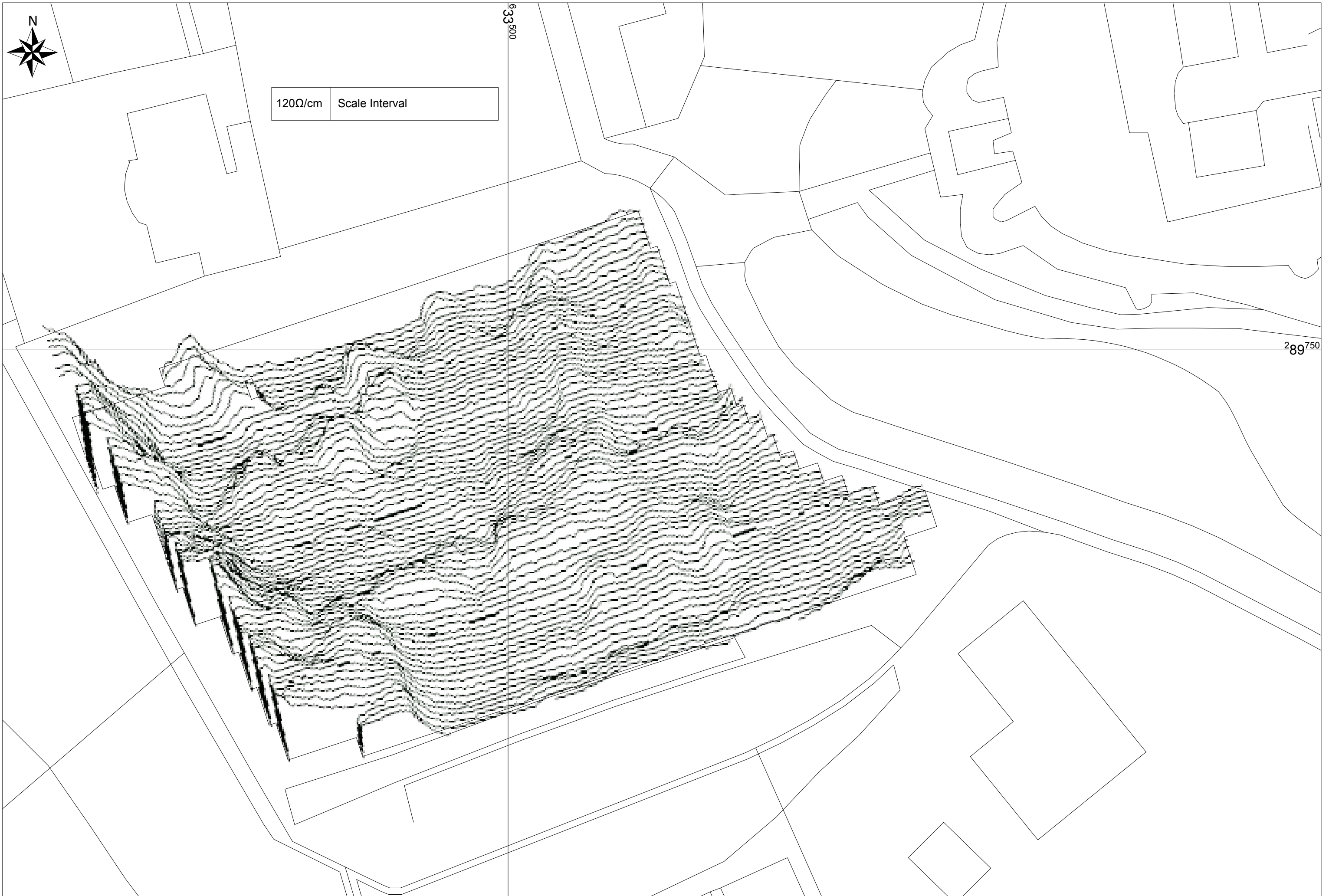
Figure 10. Processed earth resistance meter xy trace plot
