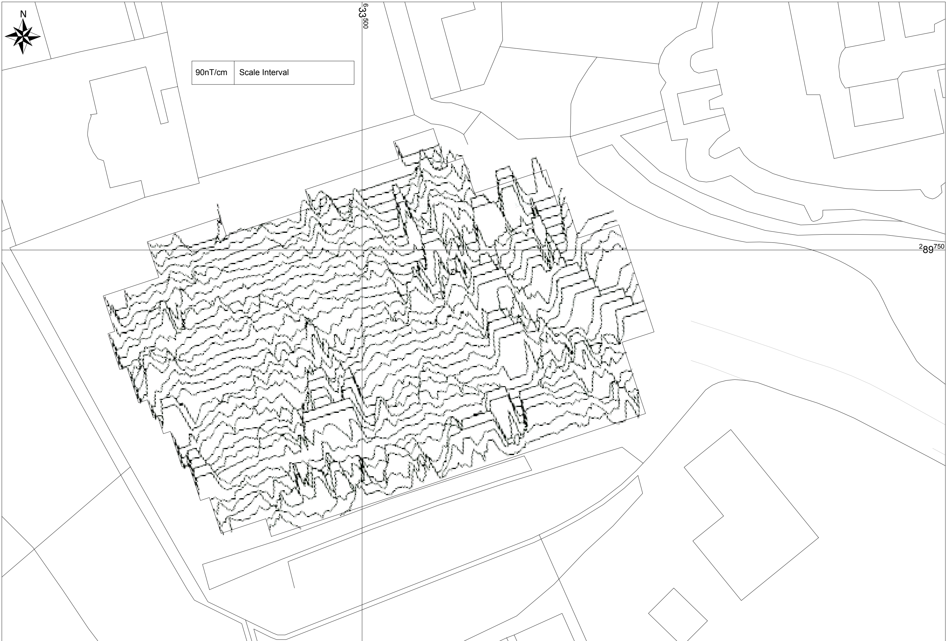
Figure 6. Processed magnetometer xy trace plot
