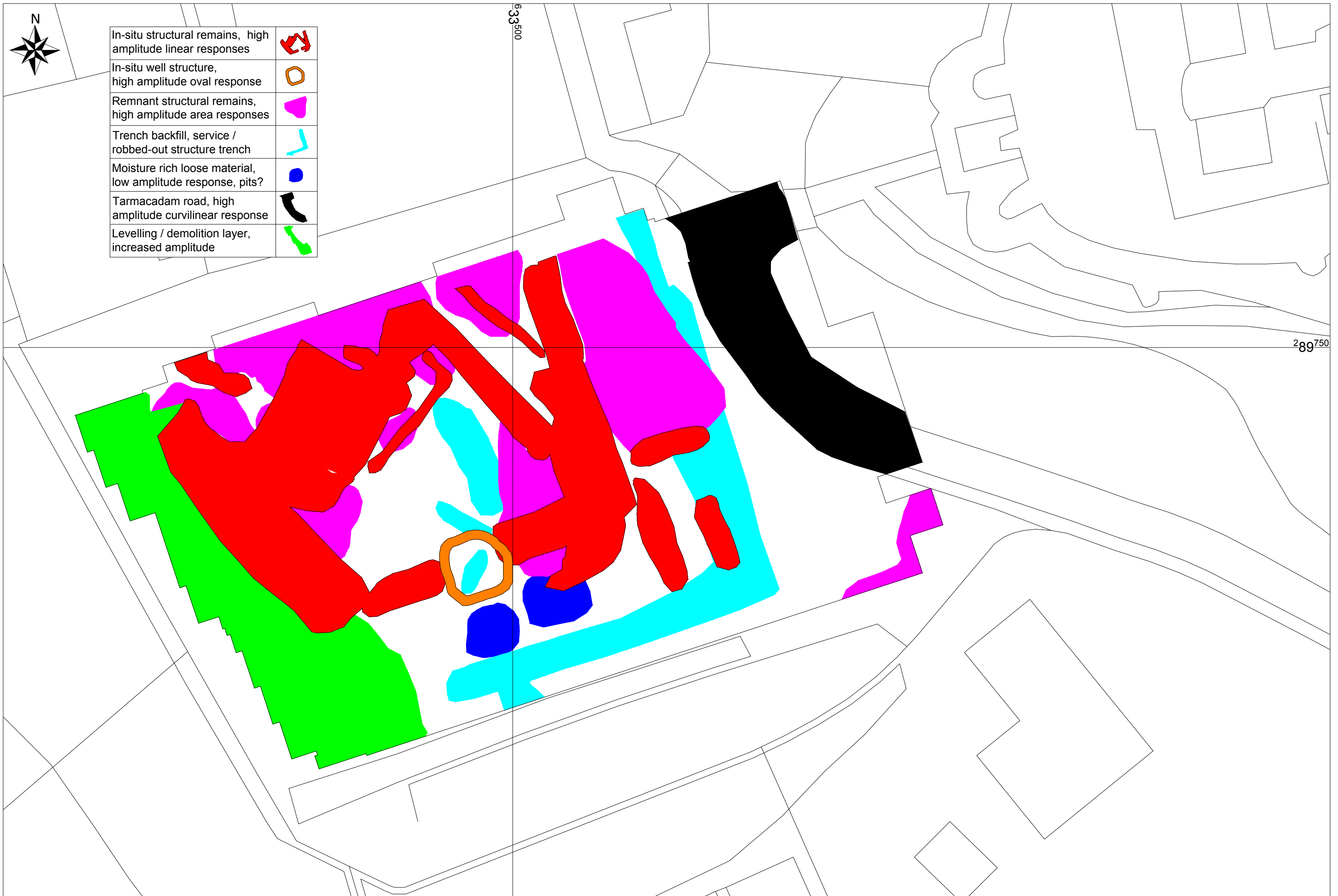
Figure 14. Combined interpretation plot of geophysical survey anomalies
