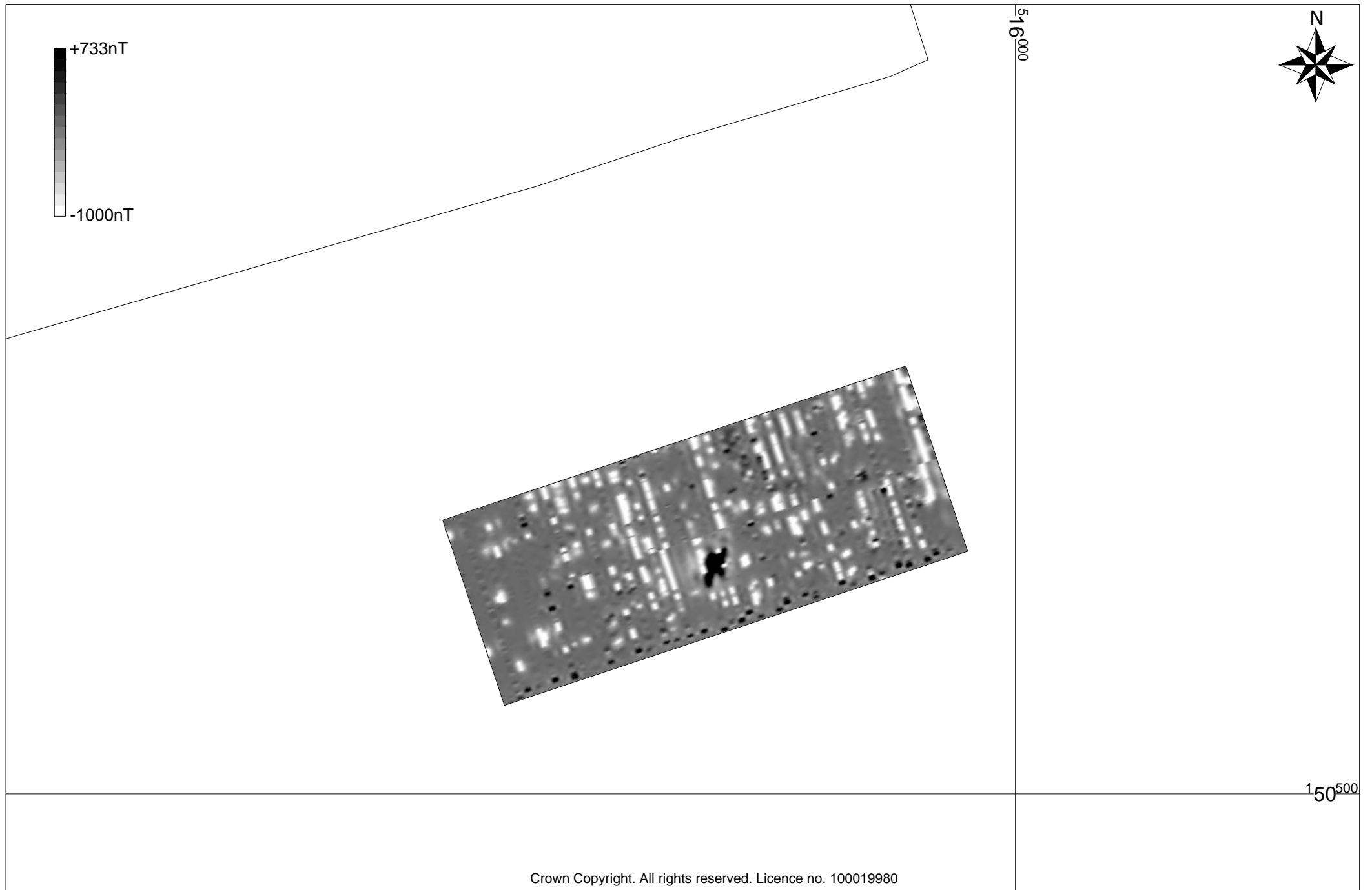
Figure 3. Raw magnetometer greyscale plot
