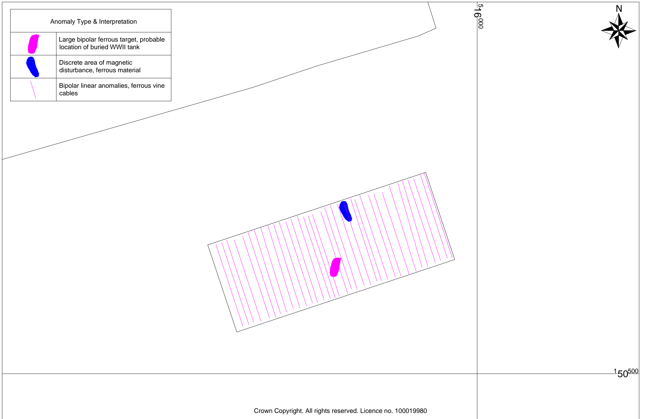
Figure 6. Interpretation plot of magnetometer anomalies
