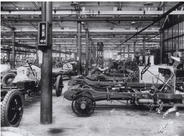
The chassis erecting shop in the main works, c.1913. (Courtesy Sir Henry Royce Memorial Foundation)
