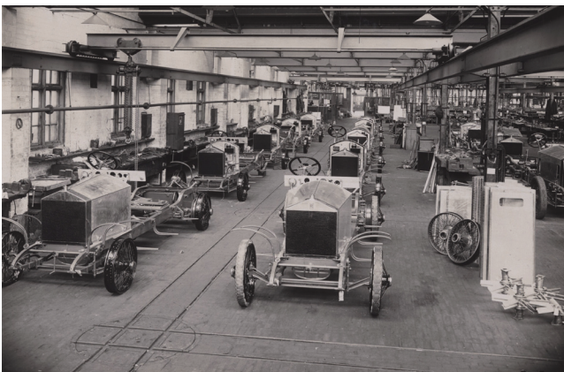
Number One shop, 1913. Note the trolley rails and turn-table. (Courtesy Sir Henry Royce Memorial Foundation)
