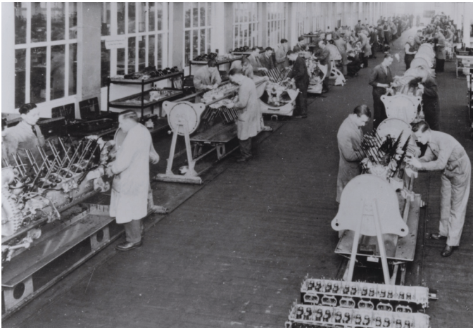
Merlin engines in production at the Nightingale Road Factory. (Courtesy Sir Henry Royce Memorial Foundation)
