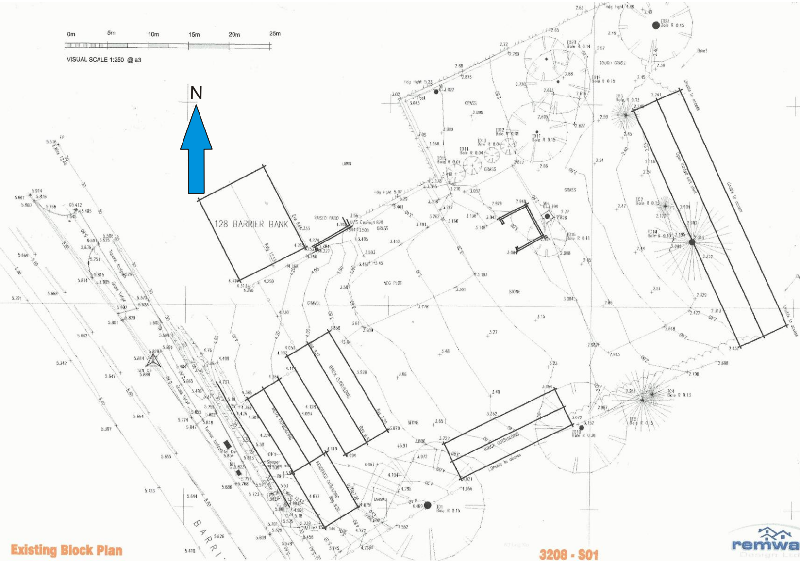
Figure 2: Plan showing the existing layout of the development site at an original scale of 1:250, (extract from Architects plan)
