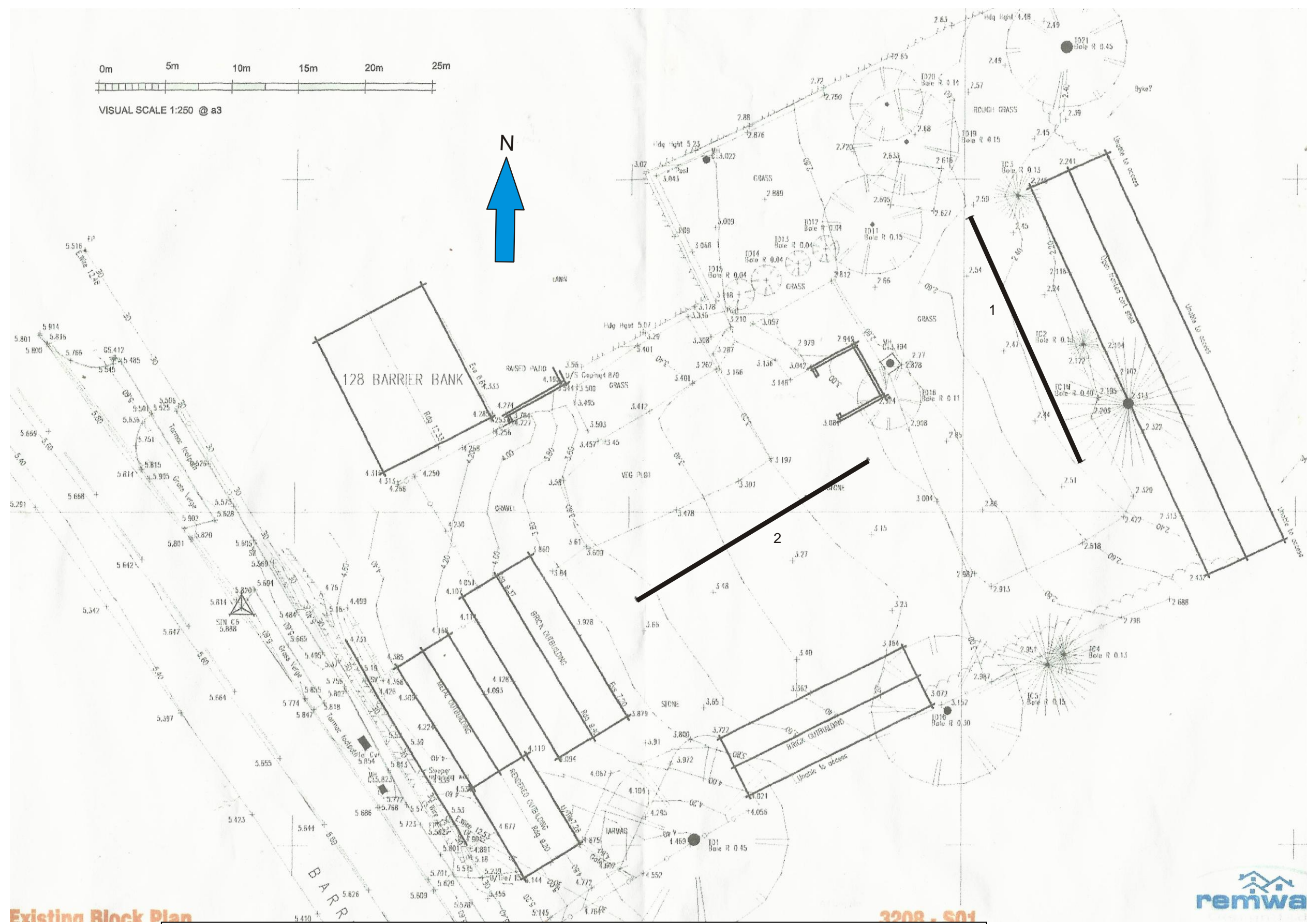
Figure 4: Plan showing the proposed layout of the archaeological trial trenches at a scale of 1:250, (extract from Architects plan)
