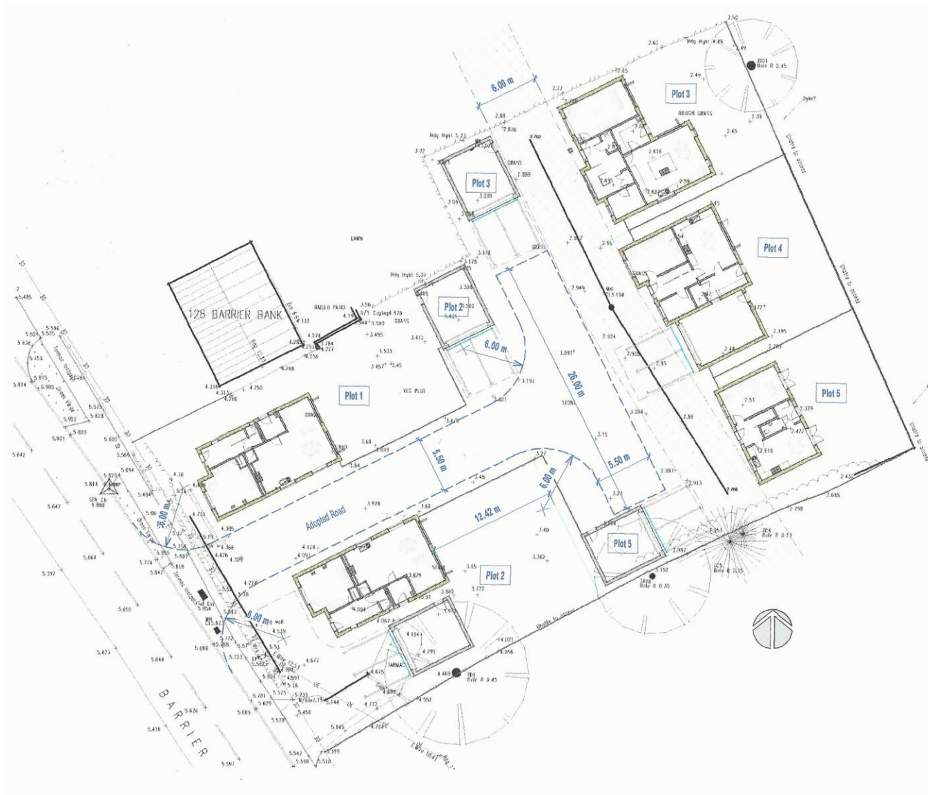
Figure 3: Block plan showing the proposed layout of the development site at an original scale of 1:250, (extract from Architects plan)
