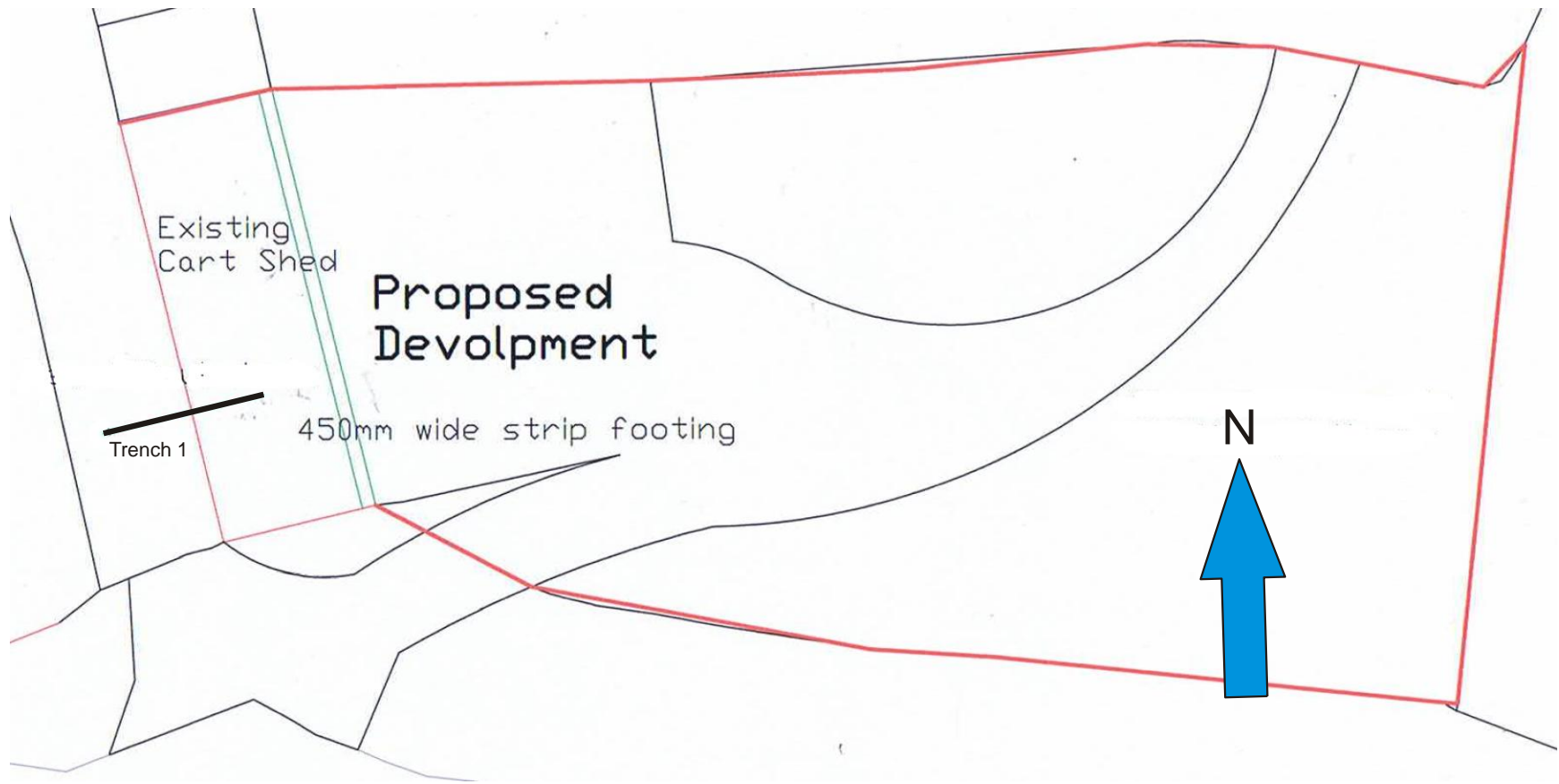
Figure 3: Plan of the proposed layout of Trench 1 , at an original scale of 1:100 (not to scale), extract from Architects plan)
