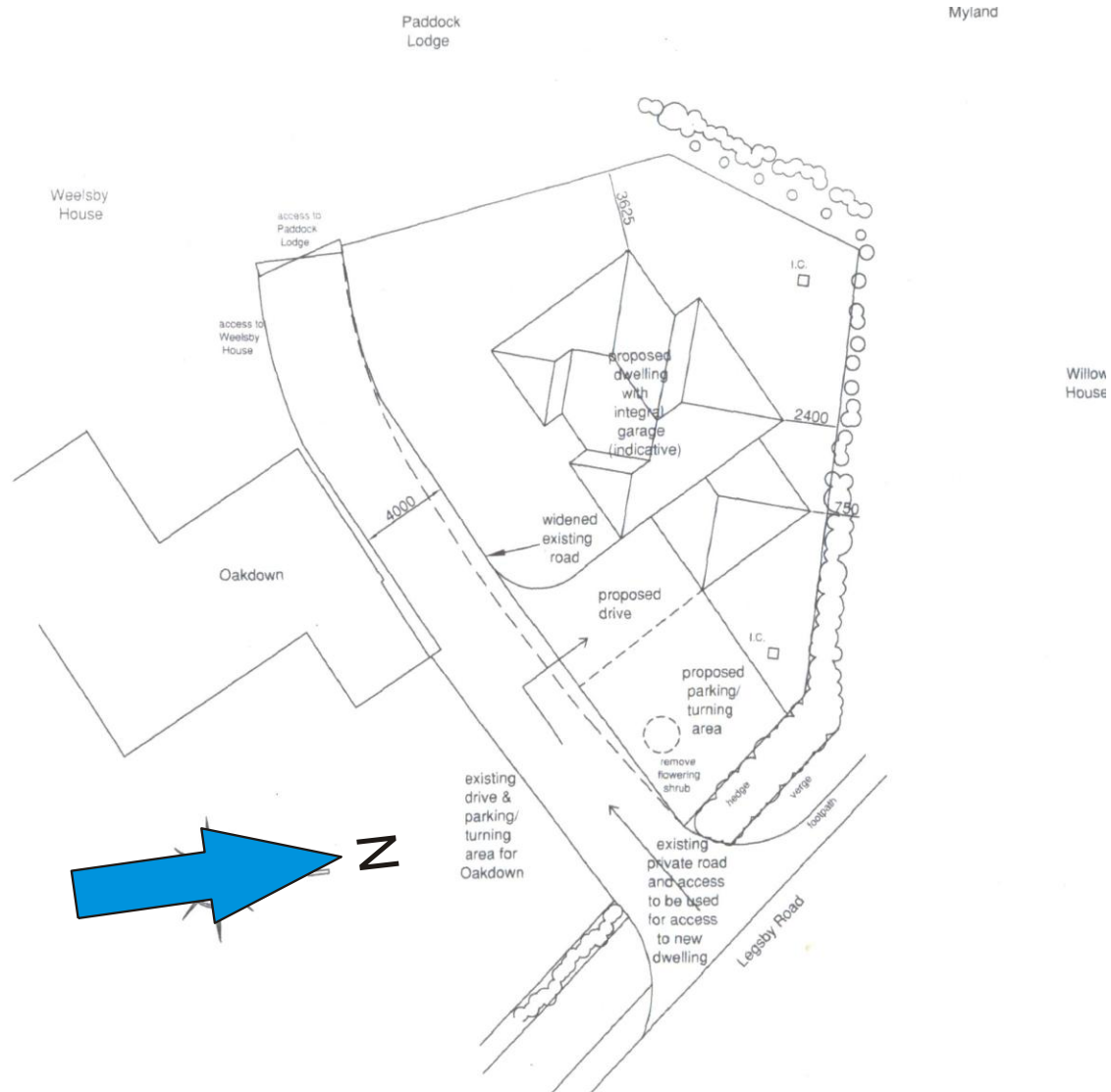
Figure 3: Block plan showing the proposed layout of the development site at an original scale of 1:200 (not to scale), (extract from Architects plan)
