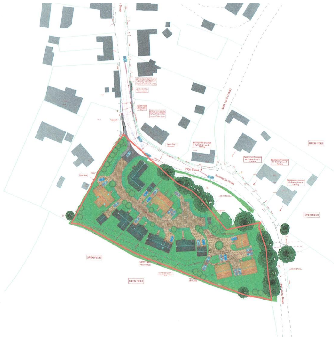
Figure 3: Block plan showing the site location and the proposed layout of the development site at a scale of 1:1,250 at A4, (extract from Architects plan)
