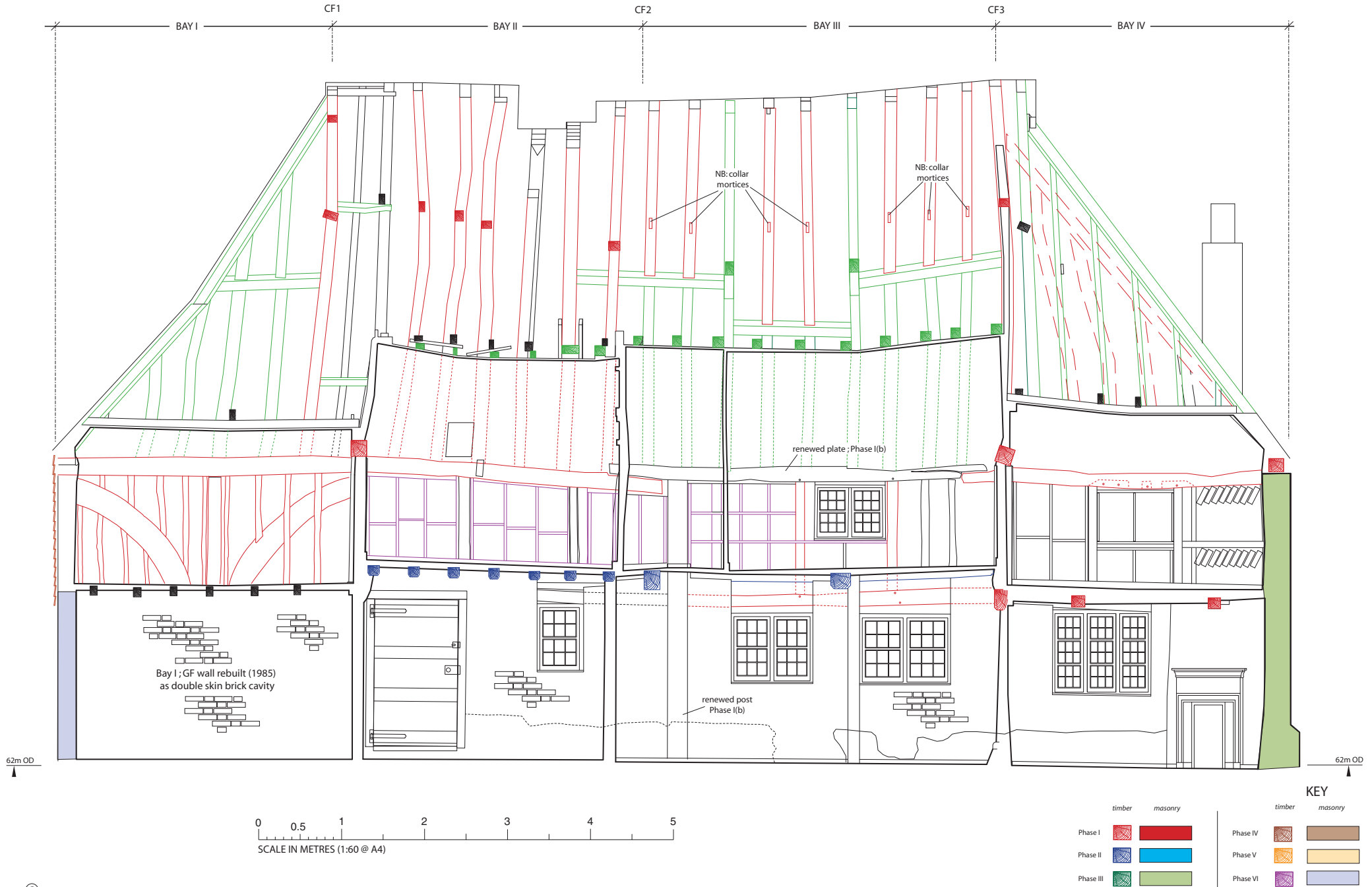
Figure 19: Interior longitudinal elevation looking south (phasing of structural elements)
