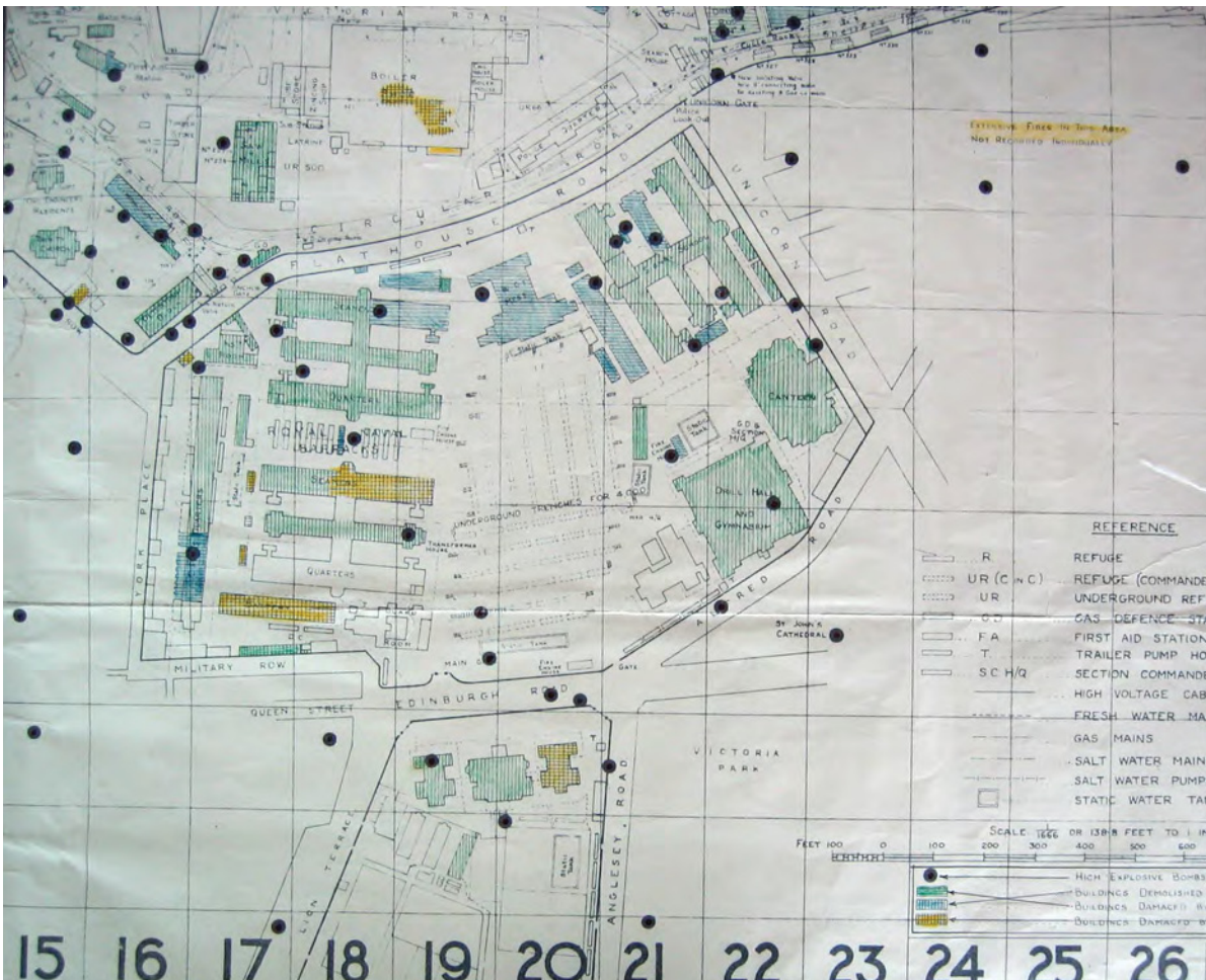
Right: Fig. 16. H M Naval Dockyard, Portsmouth: Miscellaneous. Portsmouth yard and Royal Navy barracks, showing passive defence measures, including bombs dropped and buildings damaged, 1940–43. Scale: 1:1,666. Section showing bomb falls in Area 3. TNA (1942). WORK 41/314. Reproduced with the permission of The National Archives.
