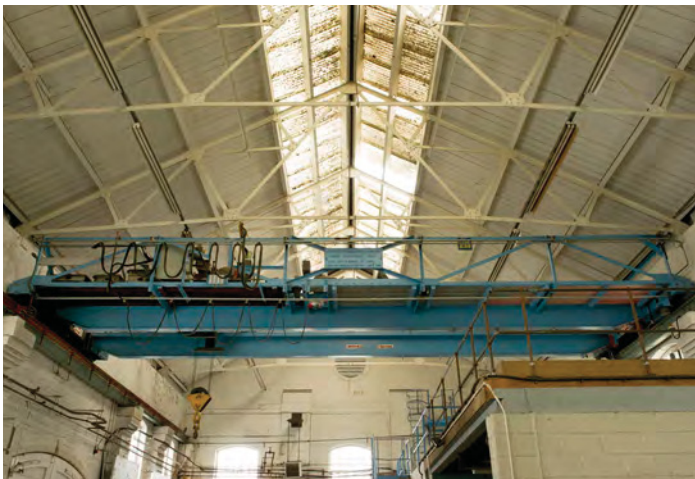
Fig. 185. DP13028. Devonport South Yard: photograph of Building S173 recorded before demolition. Interior with Cowans Sheldon overhead gantry dated 1941 (8 Feb 2011). ©Historic England.
