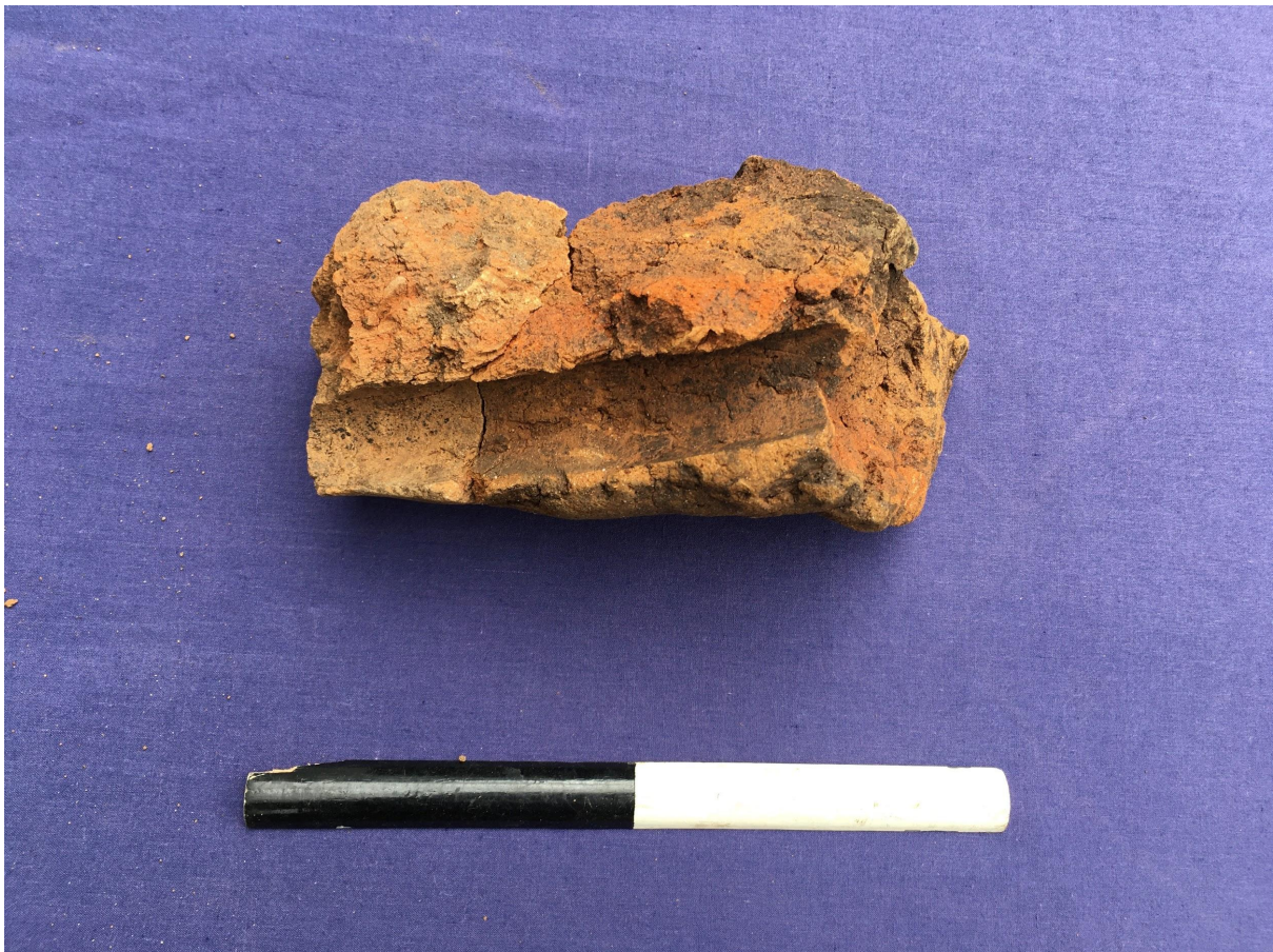
Reverse of fire bar shown in previous illustration, showing impression of a timber rod around which the fire bar had been formed. Scale 0.2m
