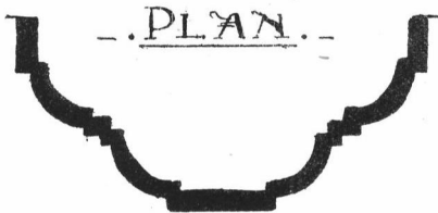
Yeardsley Hall. Oak pillar supporting the archways. Section scale \frac{1}{4} full size.
