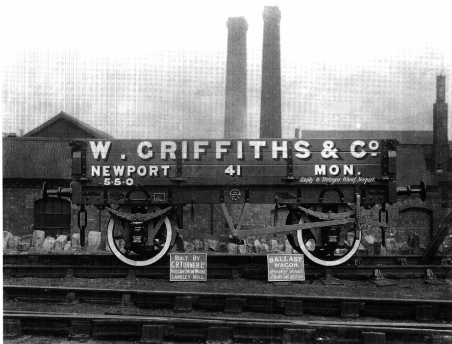
Plate 3: G. R. Turner ballast wagon with Vulcan Works beyond, 1903. Reproduced by permission of Derbyshire County Council, Derbyshire Record Office (D4156/36/1).
