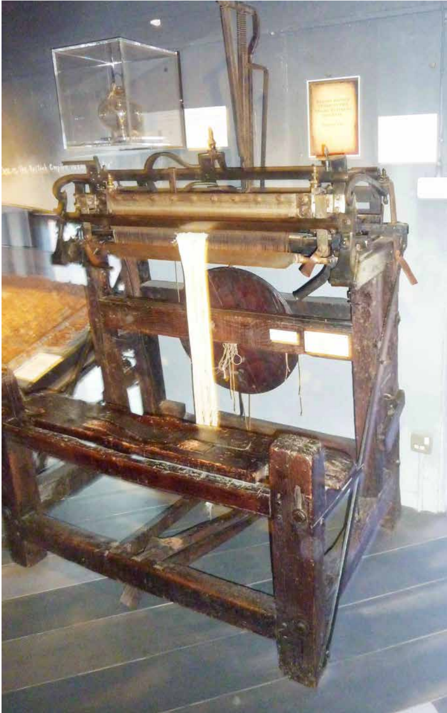
Plate 1: A framework knitting machine. This example from Calverton is in the City of Nottingham Castle Museum. On this machine two leather straps are fixed to the bench for greater comfort and ease of movement. The glass globe, top left, when hung by a window, reflected sunlight onto the frame. Similar machines can be seen in museum collections at Belper North Mill, Wollaton Hall and Ruddington.
