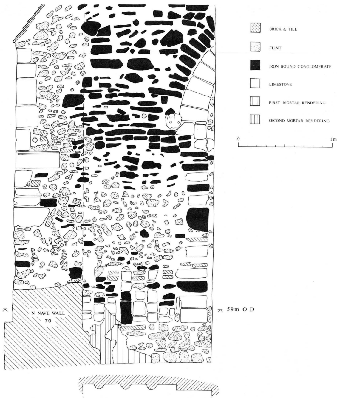
Figure 56 West elevation of nave arch, with profile of stripwork. Scale 1:25
