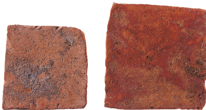
Plate 14 Ridge tile fragment T5 in a MEL fabric showing peg-hole for a crest that has become detached
