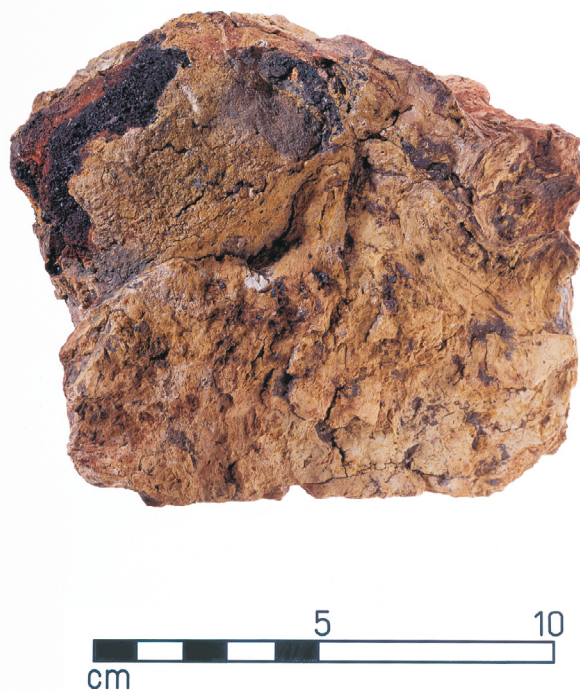
Plate 10 Refractory brick fragment showing poorly mixed fabric and massive slaggy inclusion
