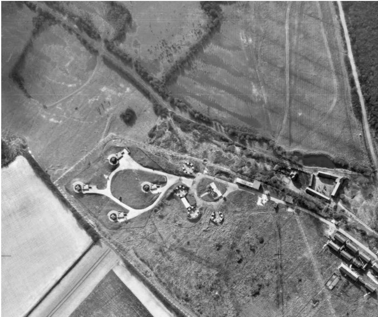
Figure 6.6 Heavy anti-aircraft battery at Bowaters Farm, Thurrock (EHER 9082). A four-gun battery with octagonal emplacements and adjacent four-gun 5.25" battery with circular emplacements which replaced the original battery in 1944. (V.82-RAF-713-pt IV-0668 held at the National Monuments Record)
