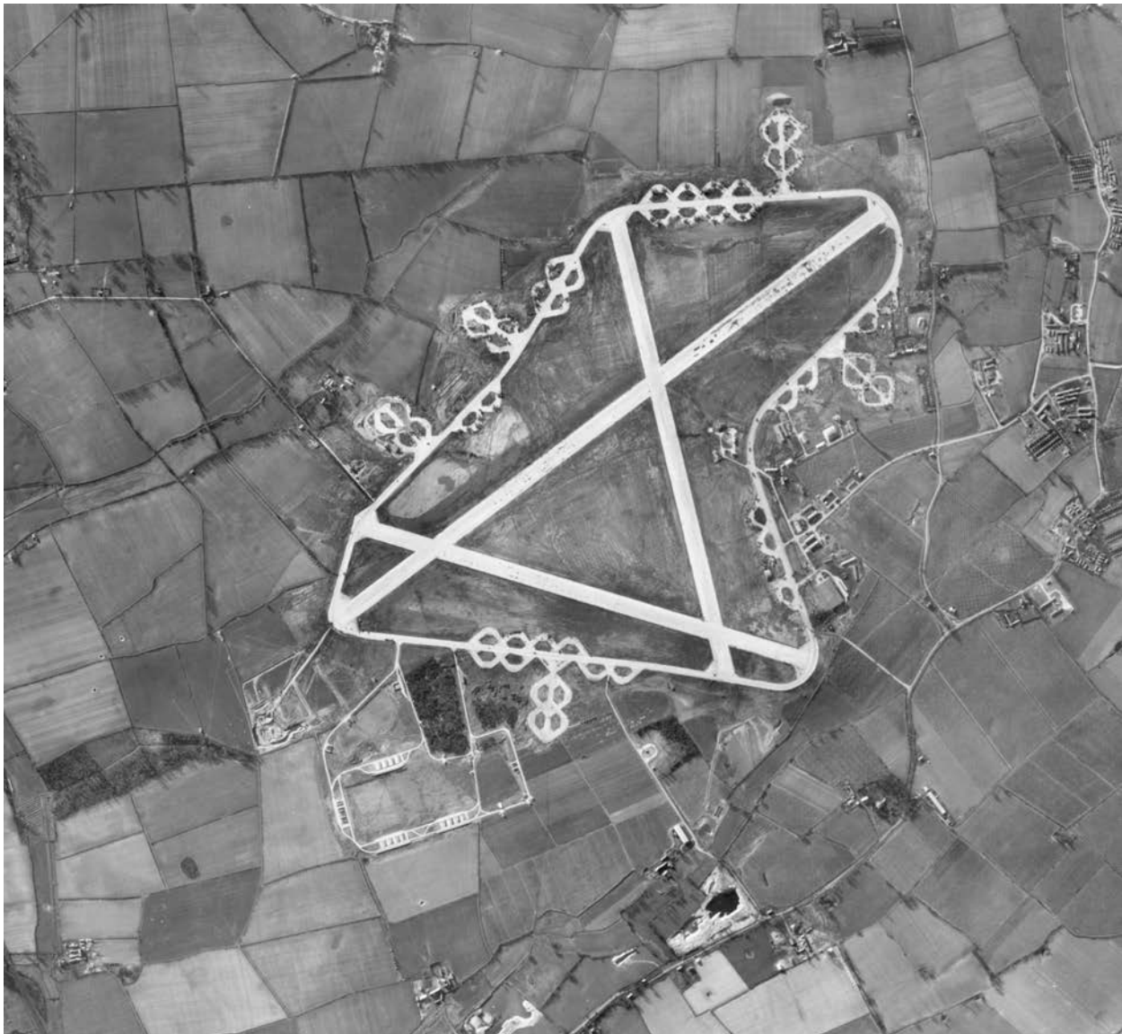
Figure 6.13 Boreham Airfield 1944: class A design with loop standings (US 7PH GP LOC 186 5013 held at the National Monuments Record)
