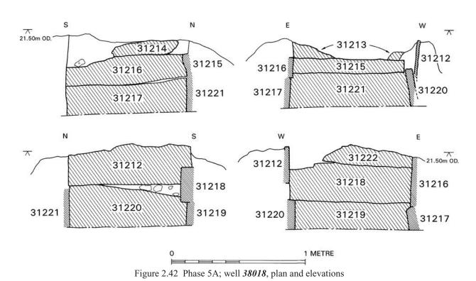
could be examined. Unusually, the lining was built solely of fast-grown, sawn green oak planks of varying width. There were no corner-posts, and the timbers had been edge-lapped together (Darrah, Chapter 8): the planks were lapped on one edge only, while there was no evidence for the use of nails. Some un-lapped planks may have been used to infill spaces
