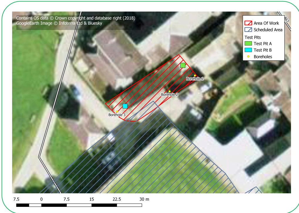
Figure 2 – Area of watching brief, showing location of geotechnical boreholes and test pits
