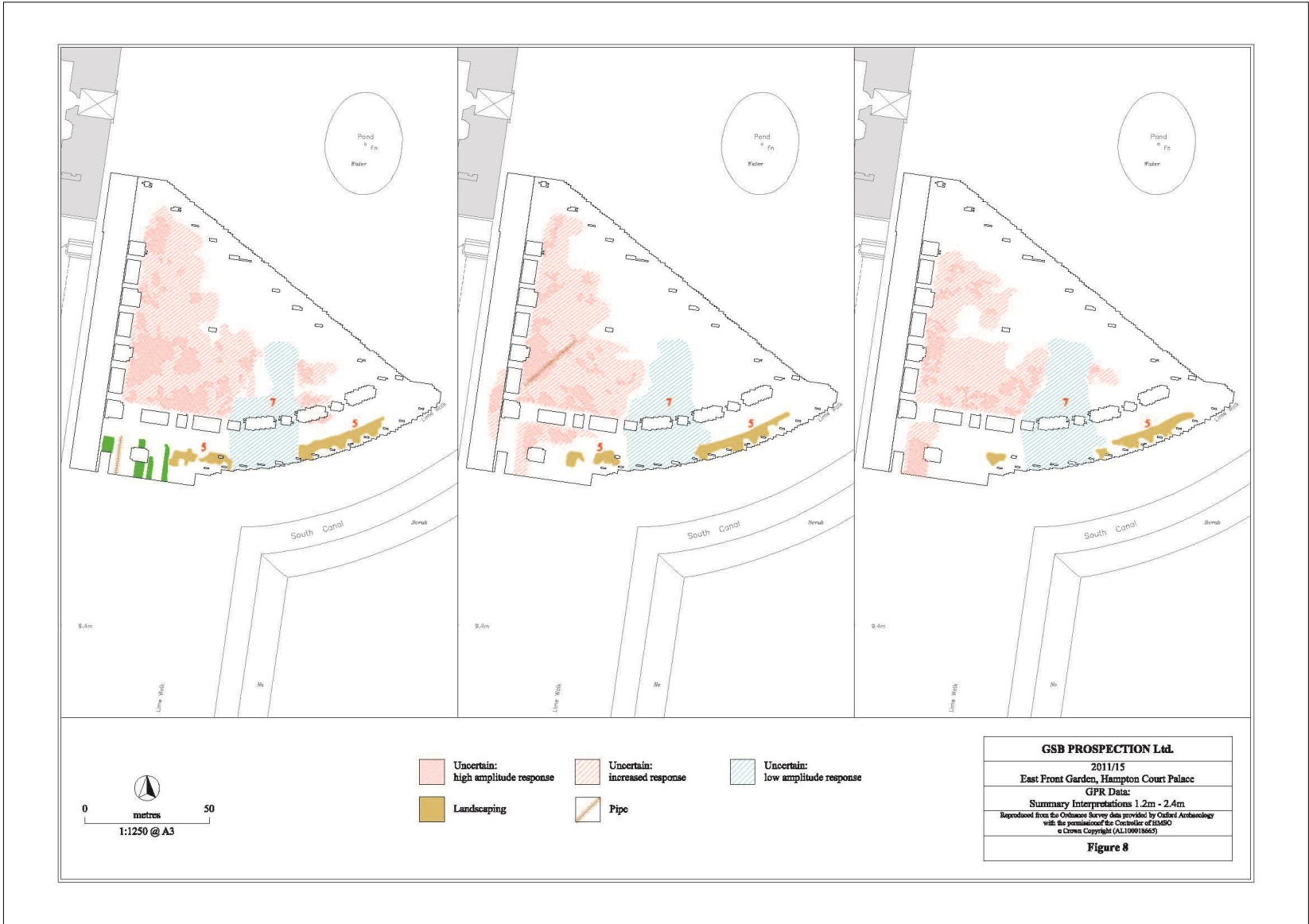
Figure 12: Plans showing the results from the GPR survey, the area of low amplitude signal is represented by the blue area 7
