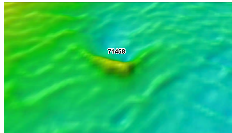
Multibeam bathymetry image of mound 71458 looking north (x6 vertical exaggeration)
