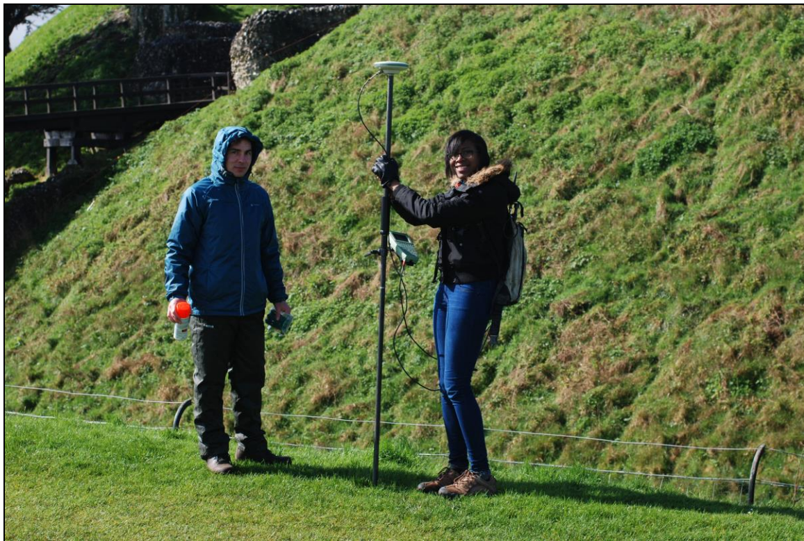
Figure 8 Leica RTK GPS with Smartnet being used to grid out at Old Sarum (photo: K. Strutt)
