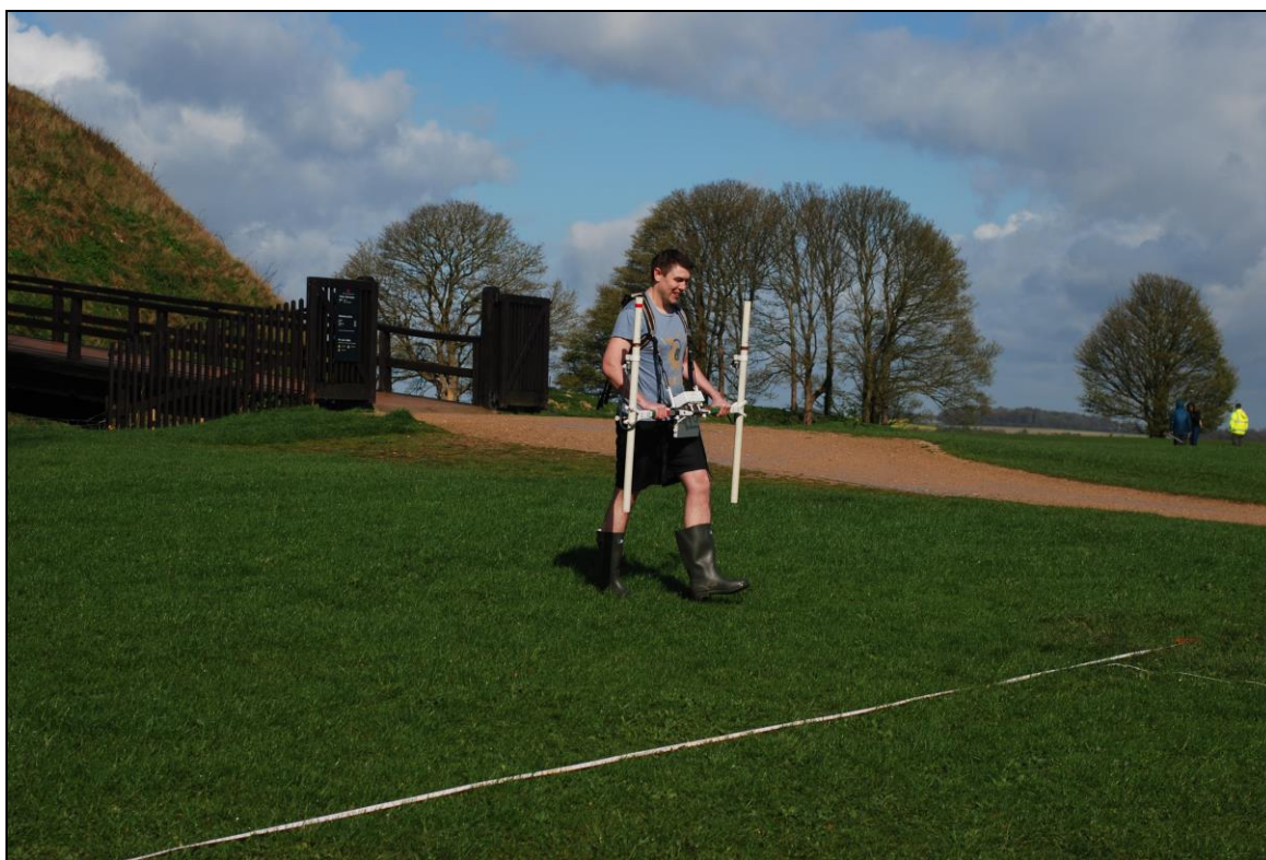
Figure 9 Magnetometer survey being conducted using a Bartington Instruments Grad 601 fluxgate gradiometer (photo: K. Strutt)
