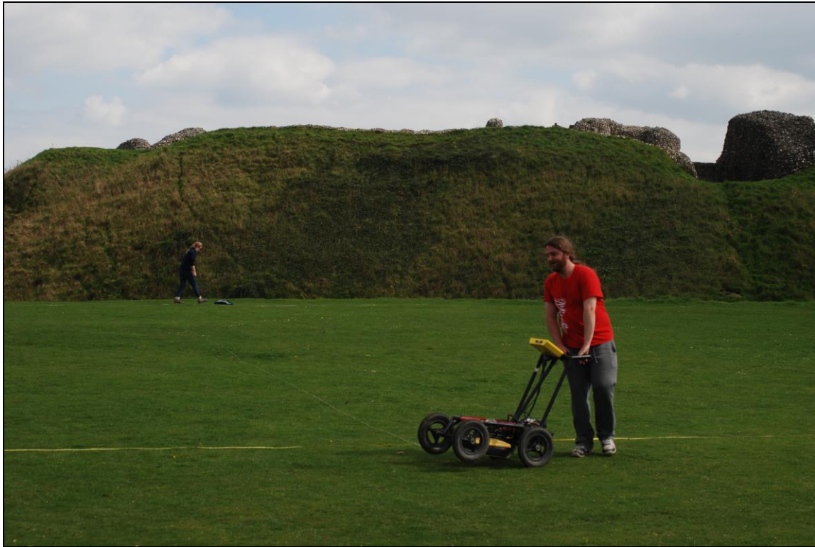
Figure 11 GPR survey being conducted in the outer bailey using a Sensors and Software Noggin Plus Smartcart with 500 MHz antenna (photo: K. Strutt)
